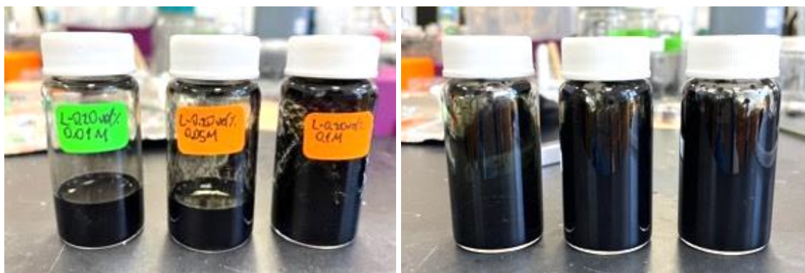
Figure 5.12. MXene dispersions of a) 0.20 vol% and b) 0.40 vol% both with 0.01 (left), 0.05 M (middle), and 0.1 M (right) NaCl.
