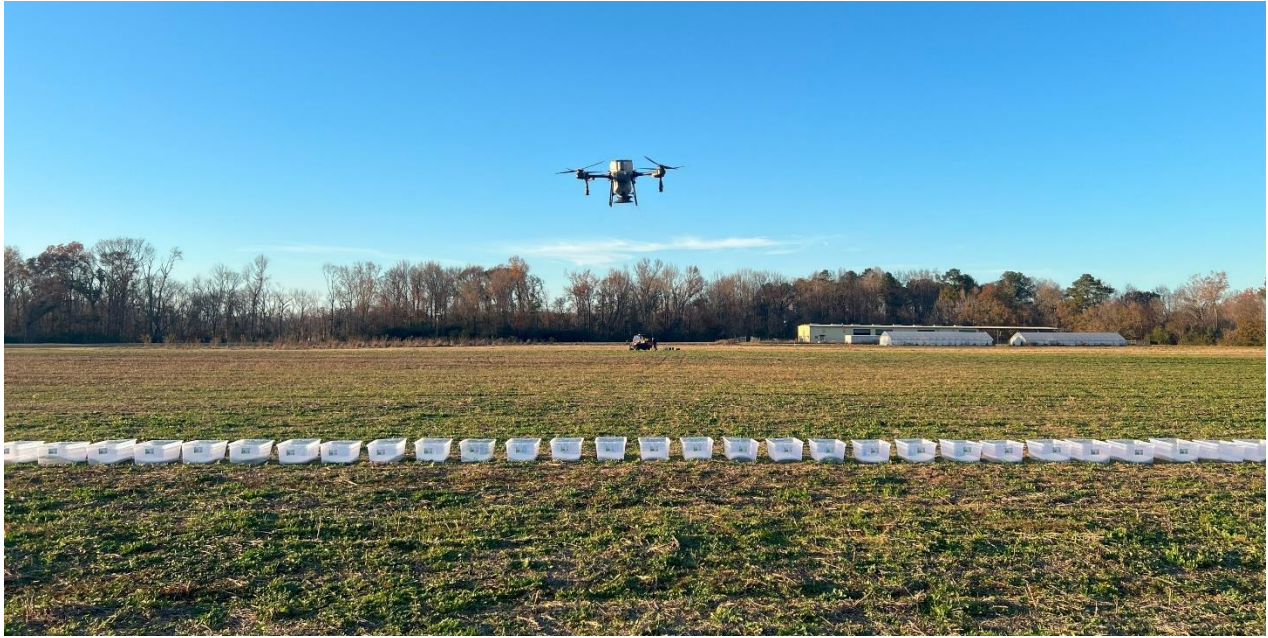
Figure 3.3. Data collection setup demonstrating the collection pans placed within the application area and perpendicular to the UAS pass for assessing the distribution uniformity of cereal rye across the swath.
