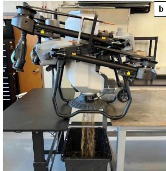
Figure 2.5. a) Materials management page on a DJI Agras controller and b) DJI Agras T25 propped between two raised objects undergoing a material calibration.
