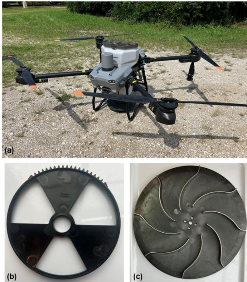
Figure 3.1. (a) DJI Agras T25 UAS equipped with the dry spreading system. (b) Large hopper (metering) gate and (c) curved-vane spinner disc used for application of cereal rye with the UAS.
