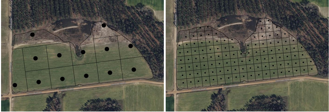
Figure 1.1. Example of soil sampling maps based on 2.0 ha (left) and 0.1 ha (right) grid sizes.
