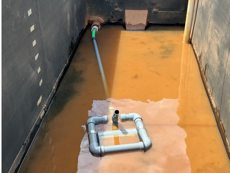
Figure 2.8 3 in. (7.6 cm) Post-Construction Skimmer Installed in the Skimmer Evaluation Tank
