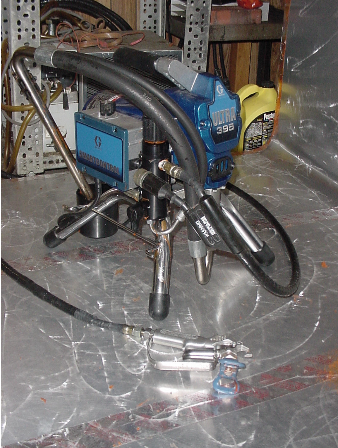
Figure 1.5-14 Test Equipment (Graco Ultra 395 Dual Action Piston Pump Paint Sprayer).
