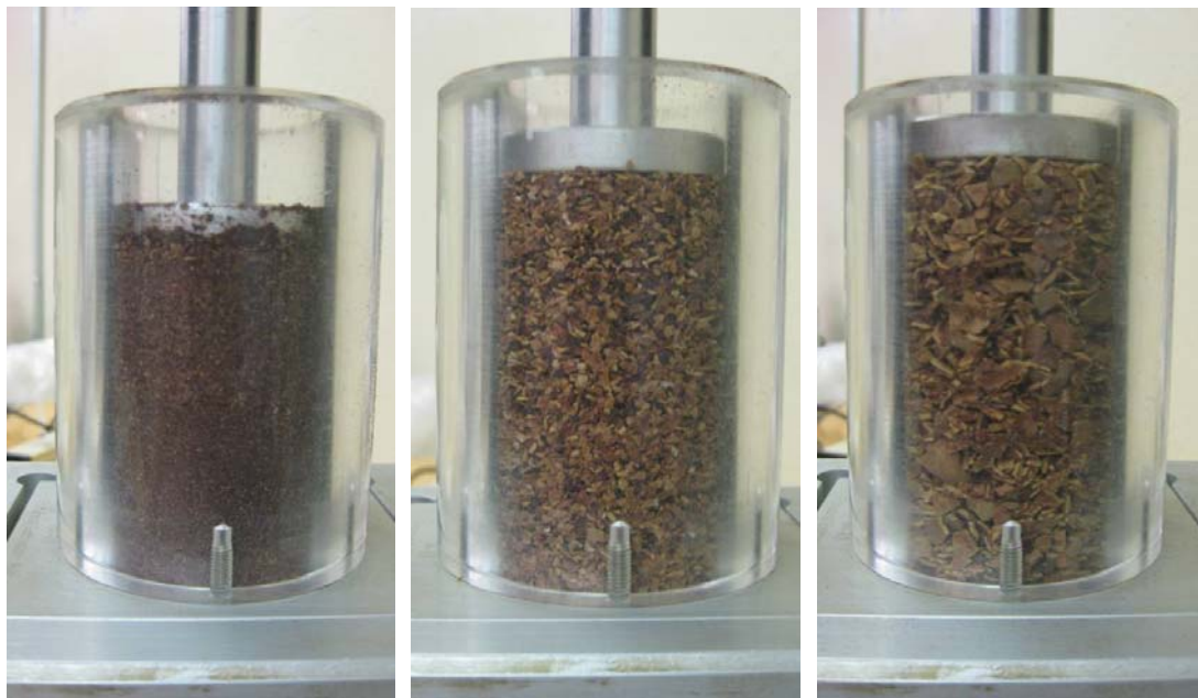
Figure D.3. Compression cell with tight fitting piston filled with fine, medium and coarse pecan shell samples (left to right)
