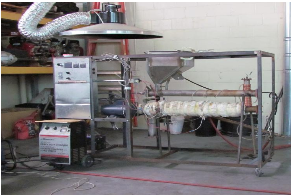
Figure E.1: Auger reactor at Auburn University used for pine wood pyrolysis in Chapter 3
