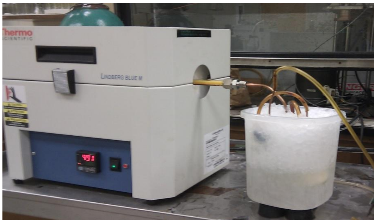
Figure E.6: Reactor set up for fixed bed pyrolysis of algae in Chapter 7
