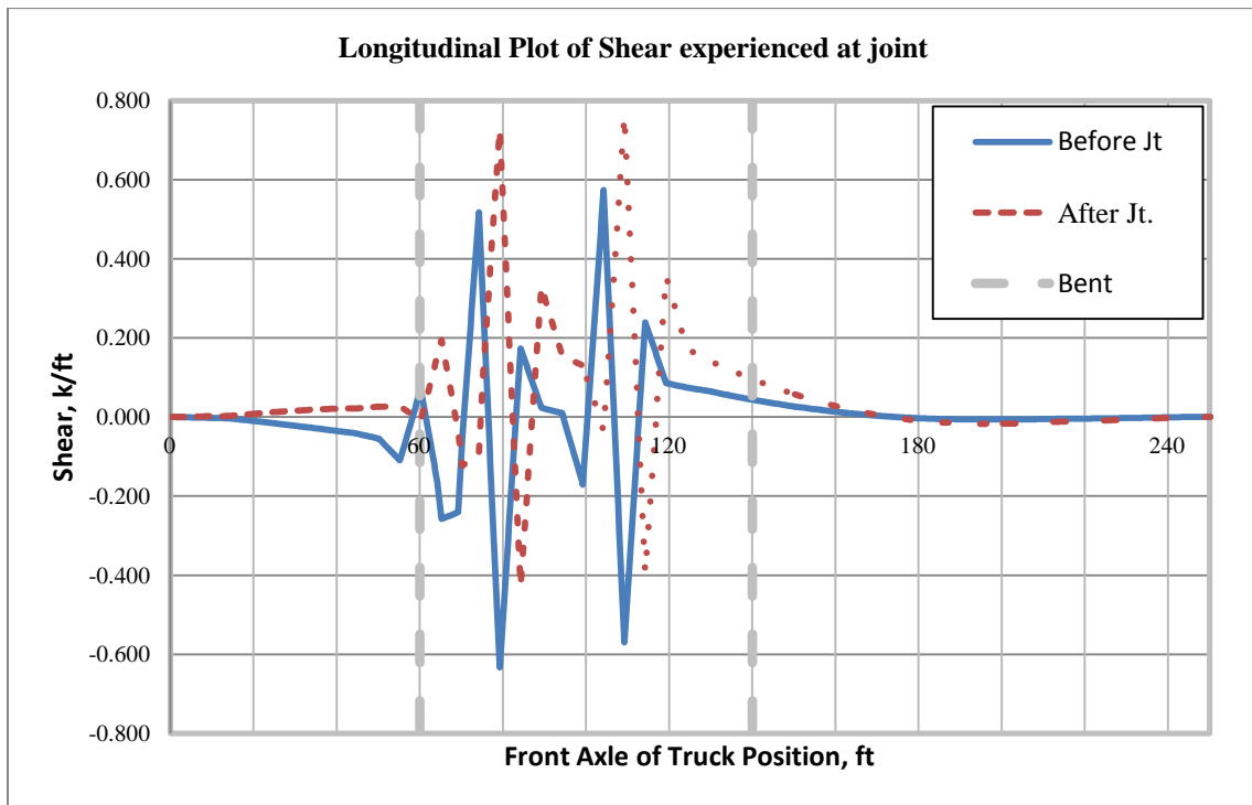
Figure 5.6: Shear Experienced in Critical Joint as Truck Passes Over Bridge
