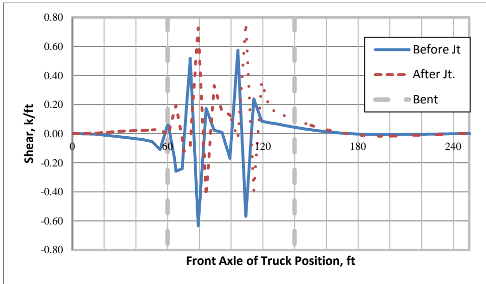
Figure 4.17: Longitudinal Plot of Shear Experienced at Transverse Position 16 as TR-13 passes (CL-2)
