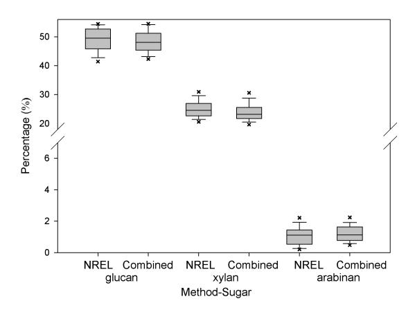
Figure 4. Comparison of variability of the monomeric carbohydrates (%) between the combined and Natural Renewable Energy Laboratory procedures.
