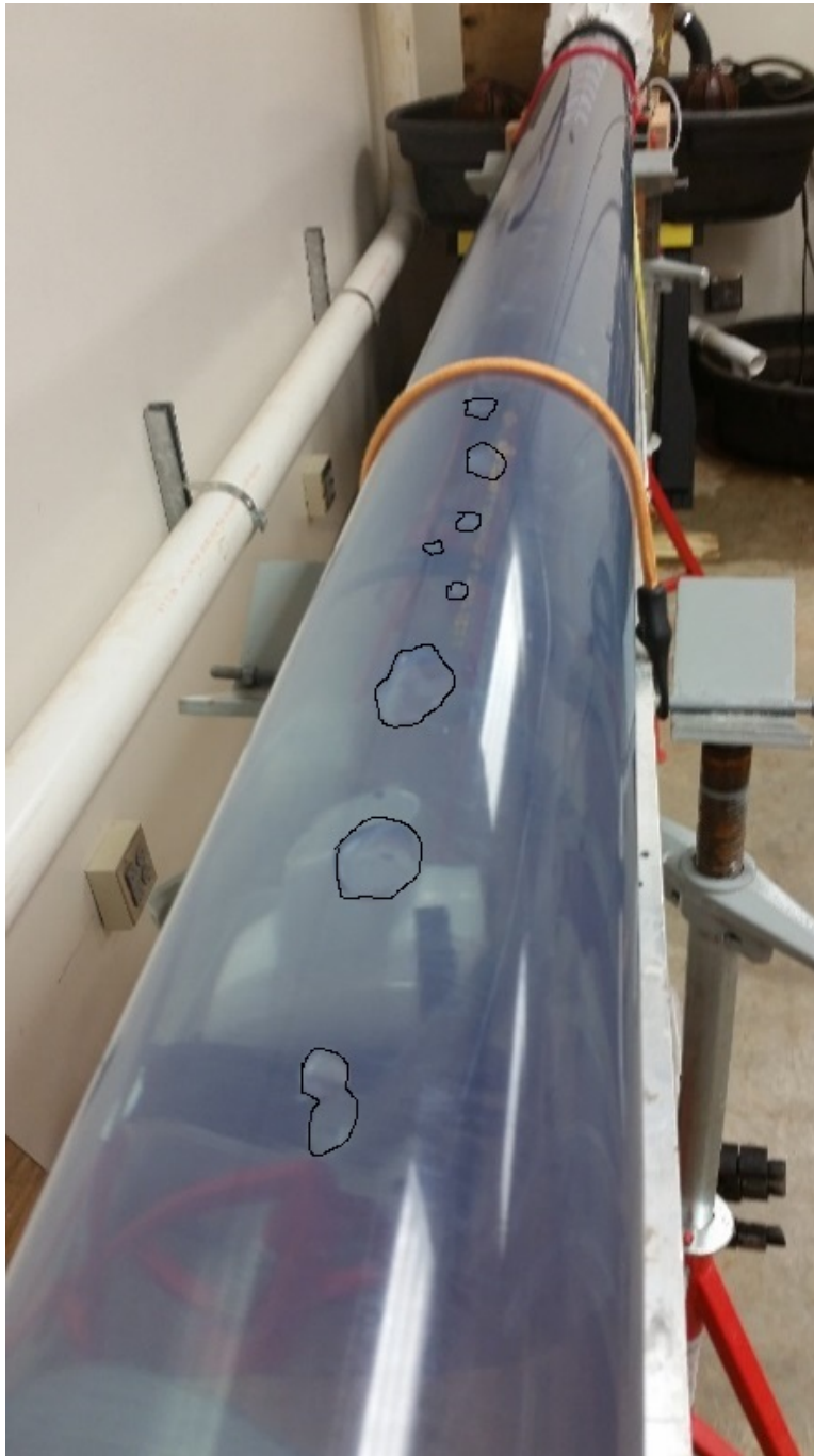
Figure 5.6: Bubbles collected along the roof of the pipe following a weak bore that caused lapping.
