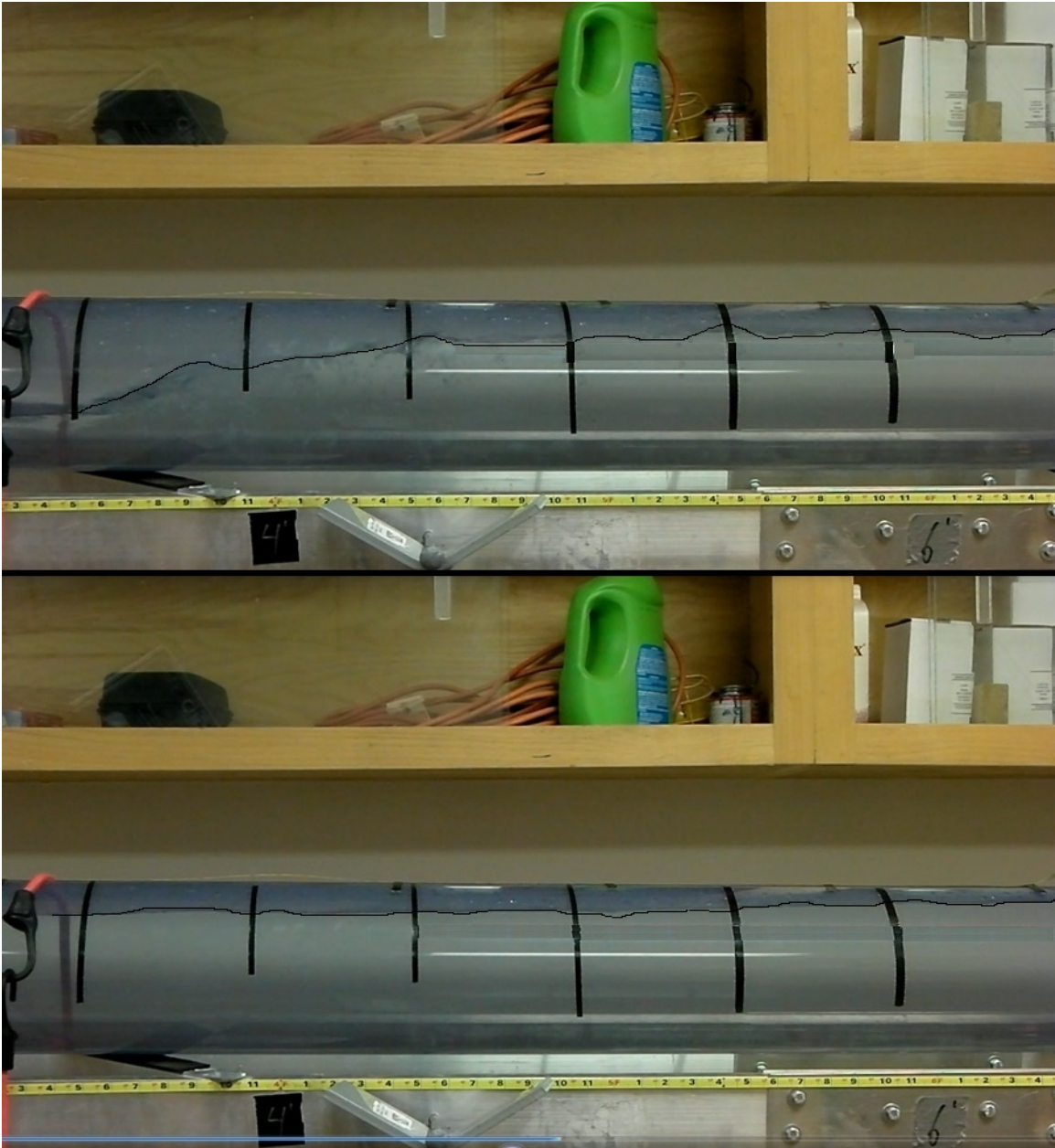
Figure 5.4: A frame taken from the camera of the case 2 bore seen in the 6 in pipe. The top image is the bore advancing and the bottom shows after the bore has passed
