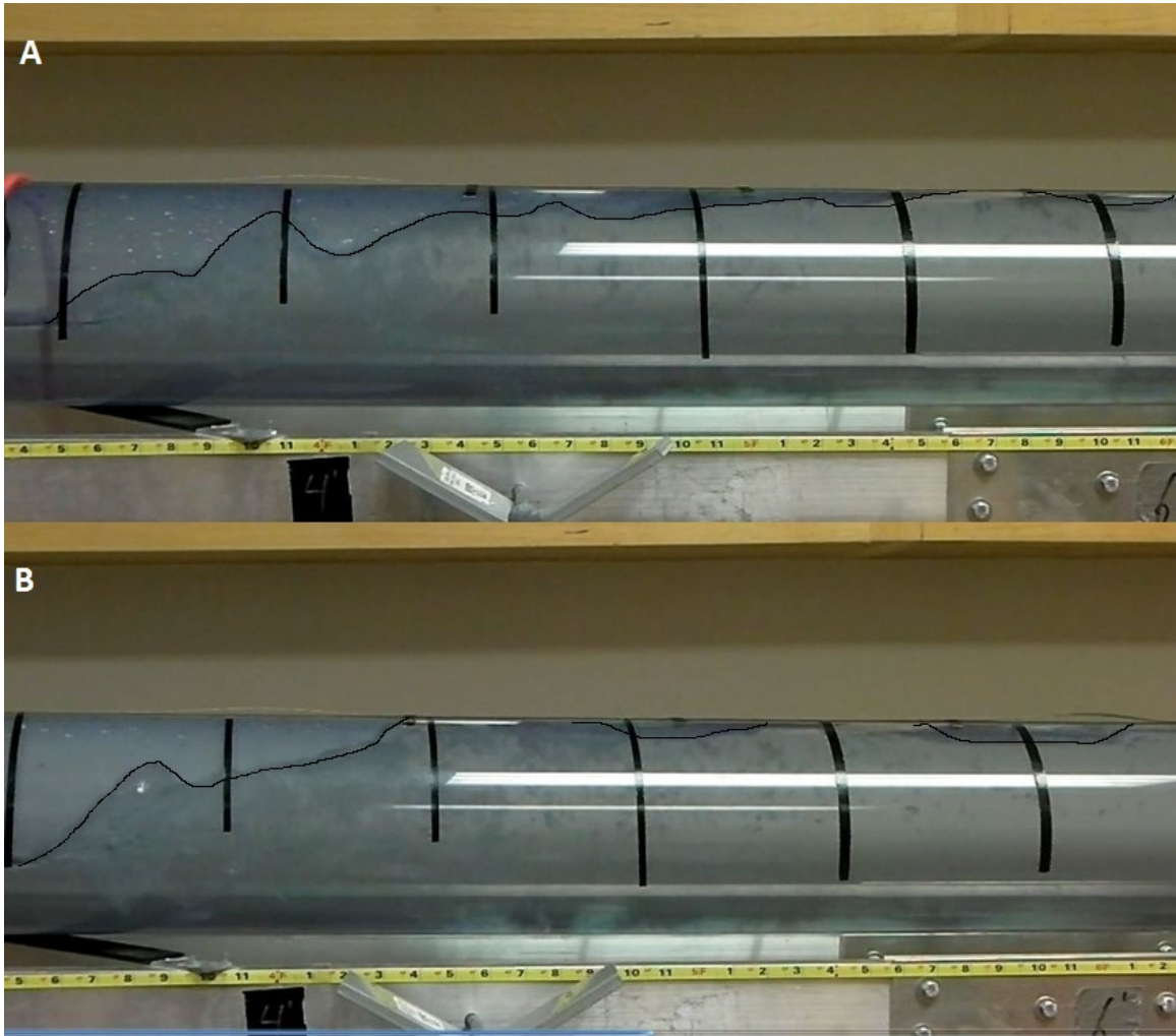
Figure 5.5: Both pipes have the same Q^* , the top image has a 1% slope with Fr. = 1.4 and the bottom image has a 2% slope and Fr. = 2.6
