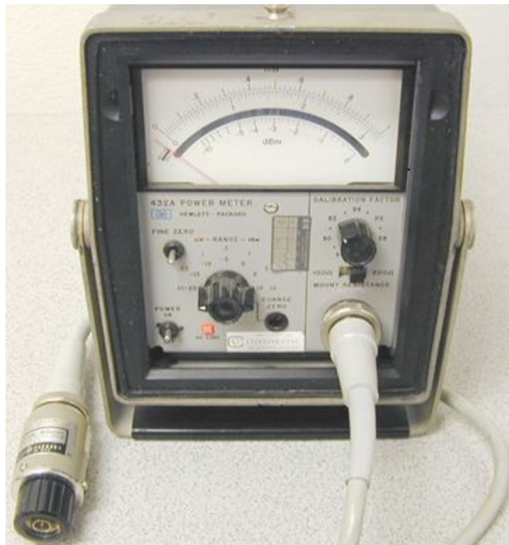
Figure B.3: HP-432A Power Meter
