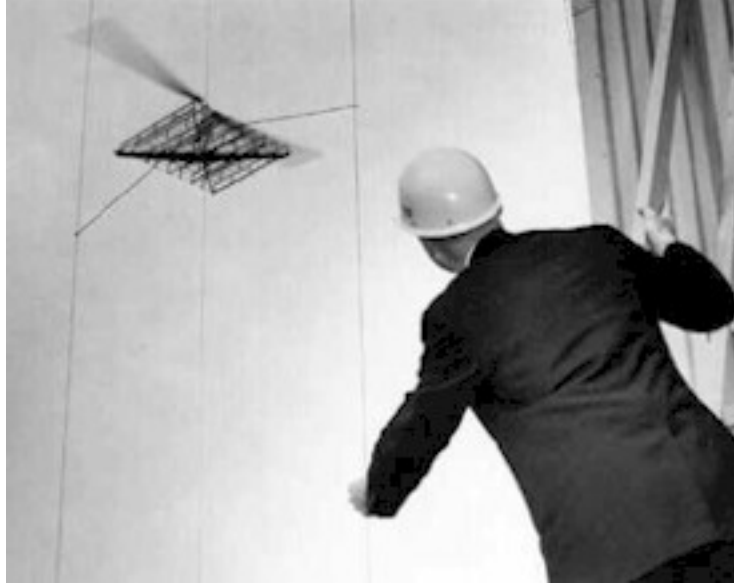
Figure 2.7: W.C. Brown's Microwave Powered Helicopter in Flight (Donchev et al., 2014)
