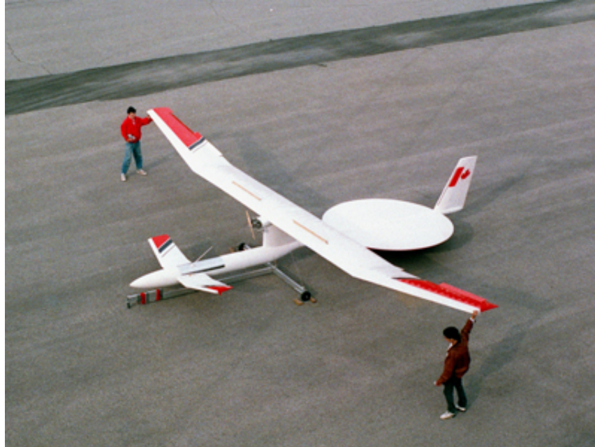
Figure 3.5: Airplane powered via a Stationary High Altitude Relay Platform (SHARP) (Wilson, 2015)
