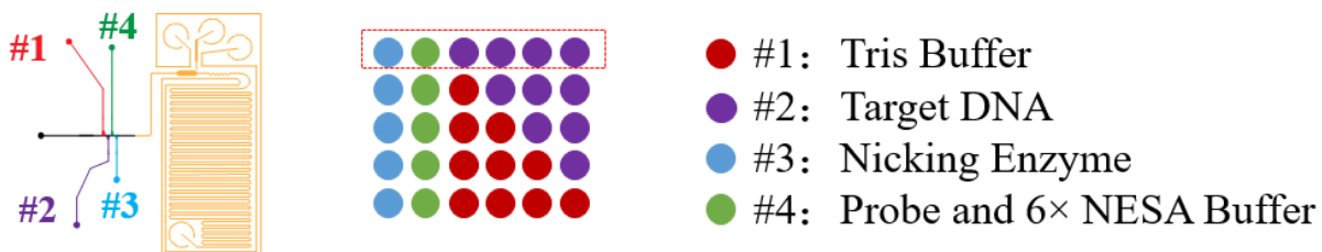
Figure 4.2 Precise, programmable reagent mixing for automated NESA with minimal reagents. Five serial concentrations of sample via progressively automatic adjusting the droplet numbers of tris-buffer and Target DNA (0-4, 1-3, 2-2, 3-1, 4-0) in this device.
