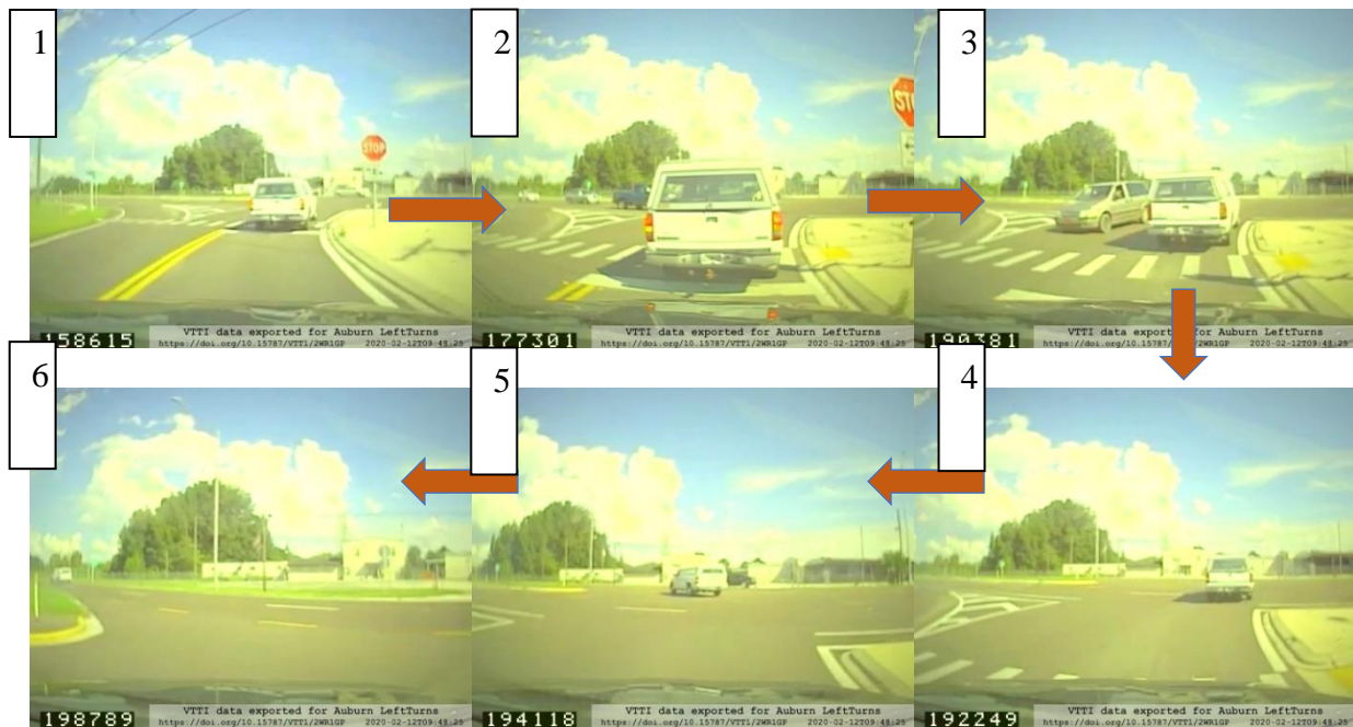
Figure 7: Time frames of a trip video showing the effect of the preceding vehicle (Frame 1: The driver sees the stopped vehicle; Frame 2: stops behind the vehicle; Frame 3 to 6: The driver starts to move following the preceding vehicle without stopping at the stop sign)
