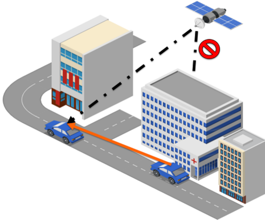
Figure 1.1: Relative Positioning with GPS Obstacles
