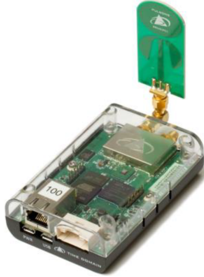
Figure 2.11: TimeDomain (TDSR) PulsON 440 Development Board [46]
