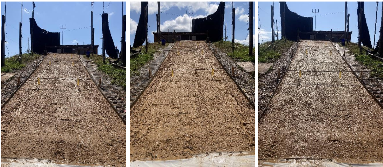
(a) after 2.0 in./hr (51 mm/hr) (b) after 4.0 in./hr (102 mm/hr) (c) after 6.0 in./hr (152 mm/hr)
