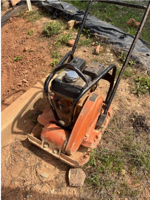
(a) plate compactor
