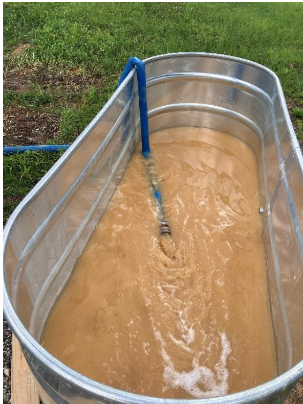
(a) tank for runoff collection
