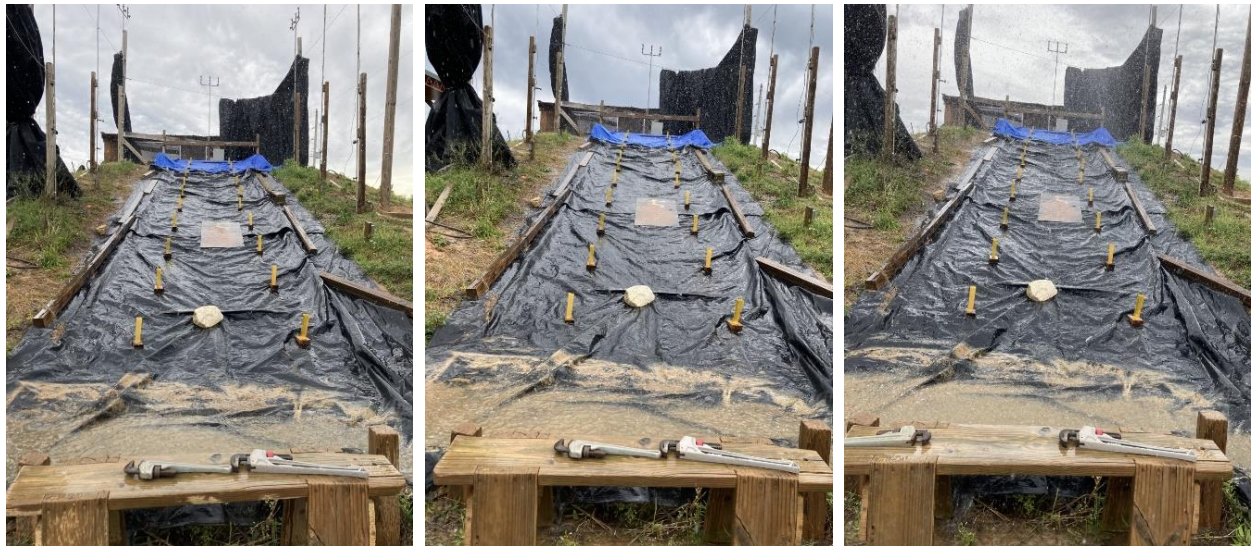
(a) during 2.0 in./hr (51 mm/hr) (b) during 4.0 in./hr (102 mm/hr) (c) during 6.0 in./hr (152 mm/hr)
