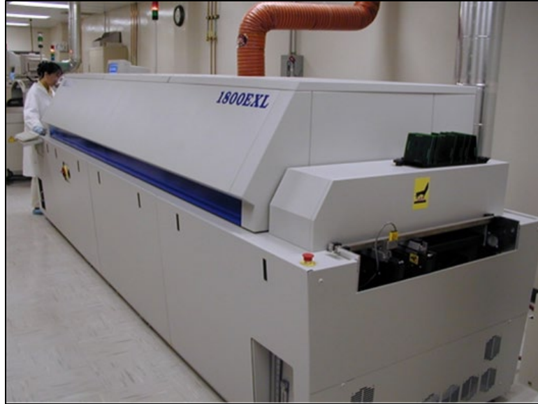
Figure 3.3 Heller 1800EXL Reflow Oven
