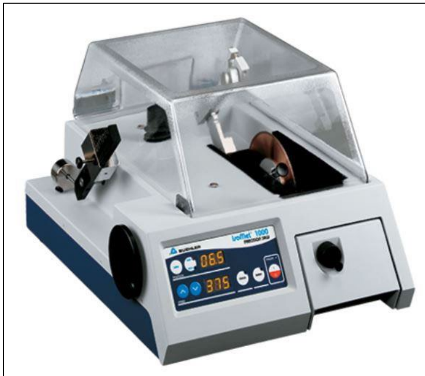
Figure 7.3 IsoMet 1000 Precision Cutter
