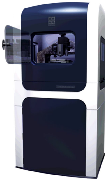
Figure 3.17 Hysitron TI950 Triboindenter
