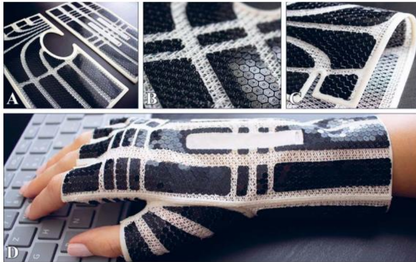
Figure 2.23. (A) Sewing pattern 3D printed using two materials, (B) surface design of glove, (C) flexible sewing pattern with inner lining, (D) pattern pieces sewn together to form a 3D printed glove [129]. (Reproduced with permission from ref. [129]. Copyright 2019 Tekstilec).
