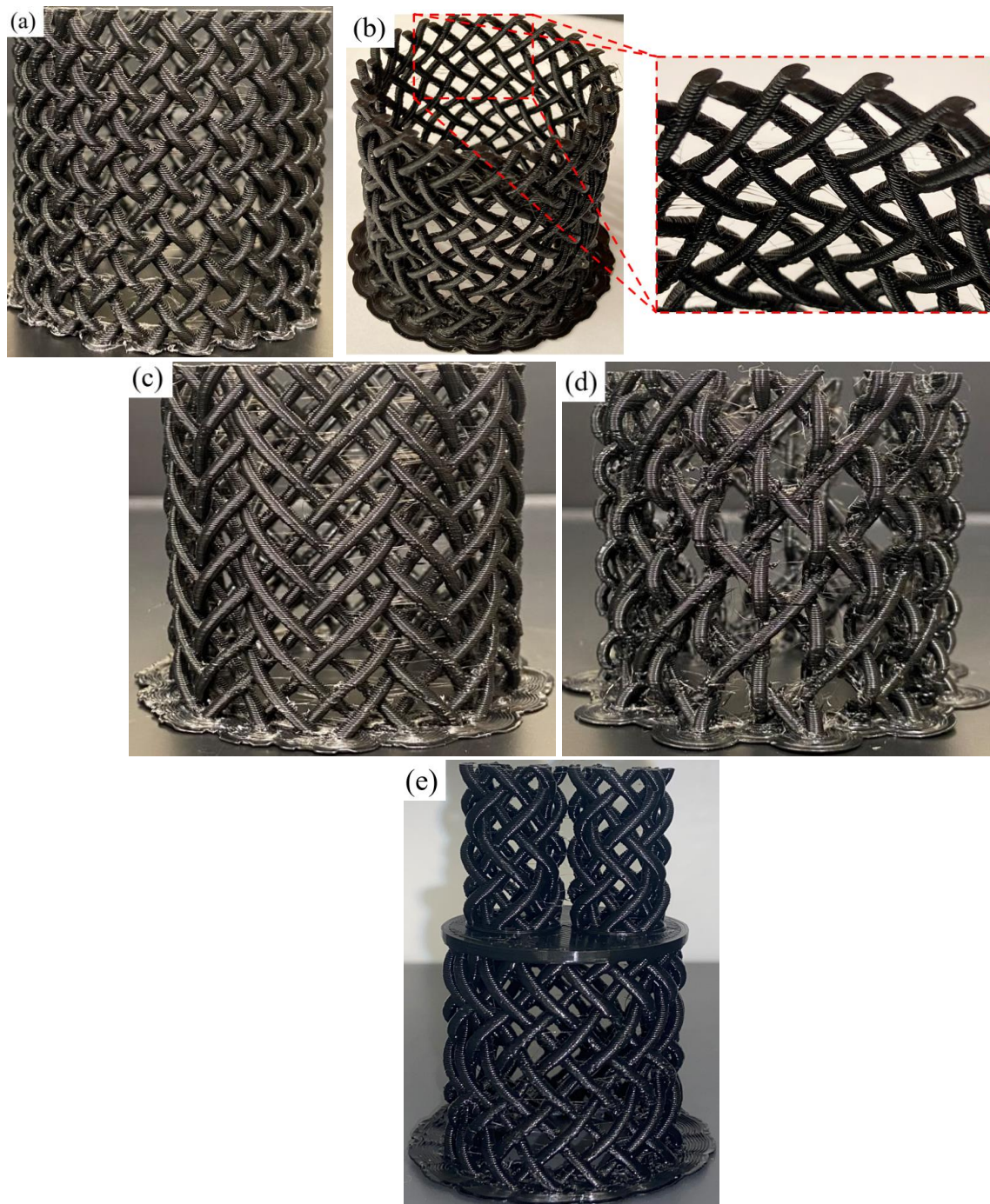
Figure 3.18. 3D printing of different designs of braided structures made of PLA. (a) Diamond braid, (b) Regular braid, (c) Hercules braid, (d) Triaxial braid, and (e) Bifurcated braid.
