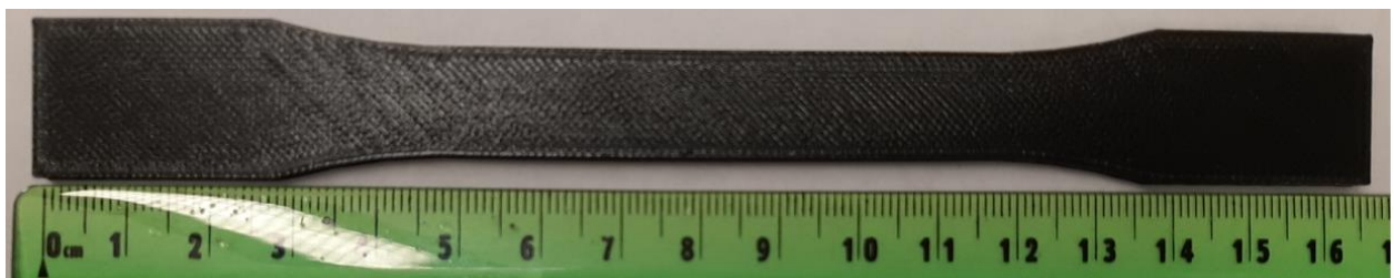
Figure 4.6. 3D printed and non-heat-treated dog-bone specimen.
