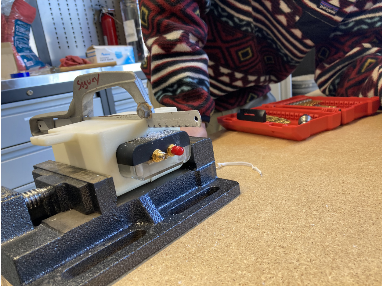
Figure B.23: Removing a UWB unit from its mounting hardware.
