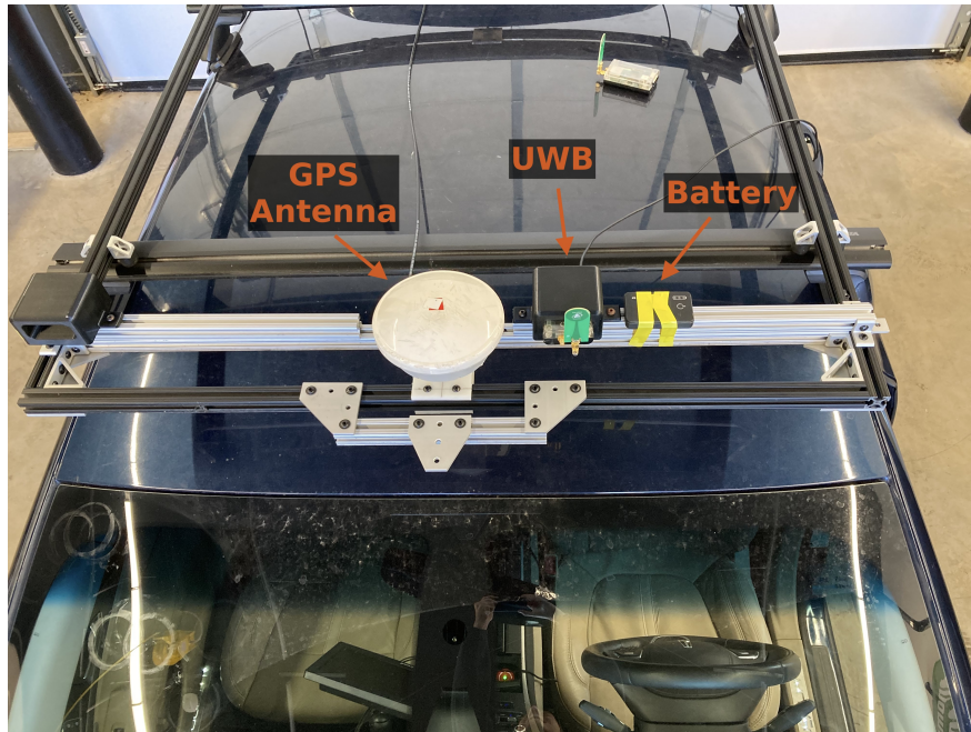
Figure 8.1: MKZ roof-mounted test equipment.
