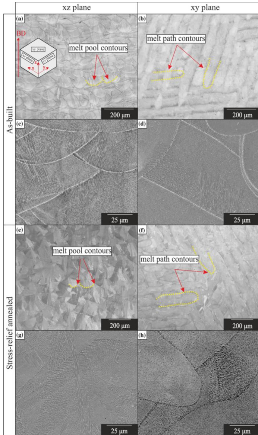
Figure 9: Optical and SEM images of (a-d) as-built IN625, and (e-h) stress-annealed LPBF IN625 [23].
