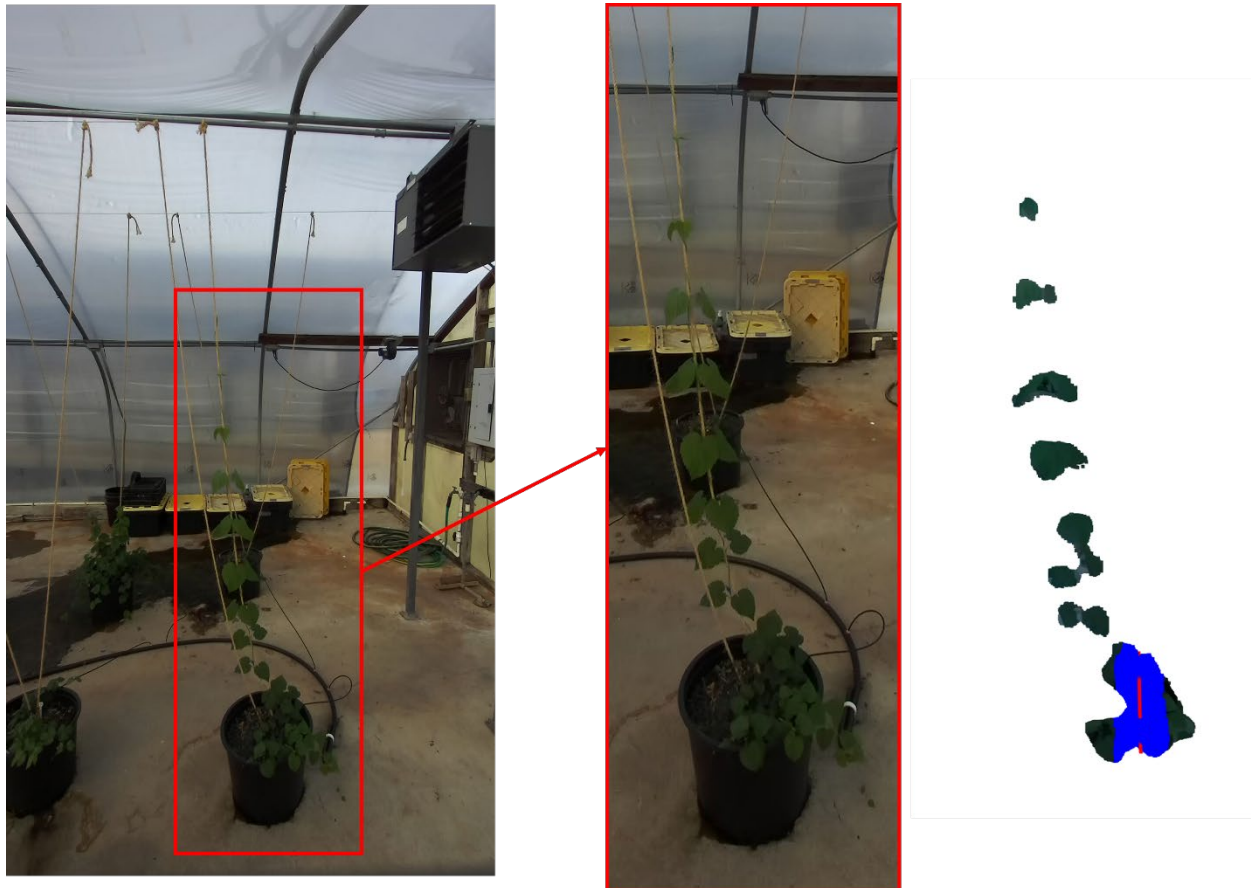
Figure 3.7 Plant 8N imaged on December 03, 2021. Measured and RANSAC derived vine length were 1.753 m and 0.347 m, respectively, for a difference of 1.406 m. Line fitted by RANSAC is in red and inliers are in blue (right). Note, plant material below 240 mm was removed in the segmented point cloud.
