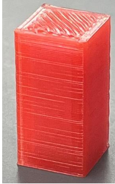
Figure 8. FFF Printed part with two voids inside.
