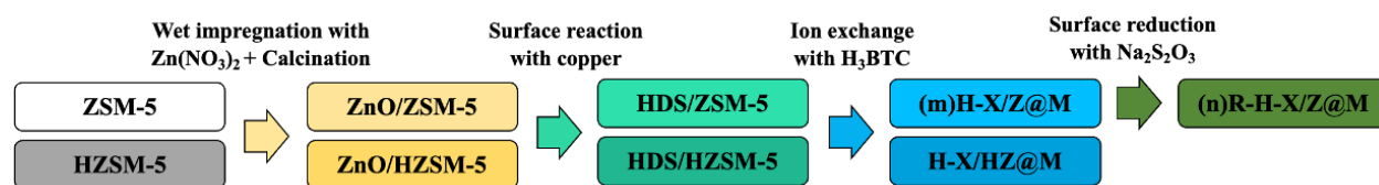
Figure 4-1 Overall synthesis process of ZSM-5@MOF-199 composites. X identifies the ligands of copper sources: nitrate (N), chloride (Cl), and acetate (A). m and n show loading of ZnO and mass of Na 2 S 2 O 3 , respectively.
