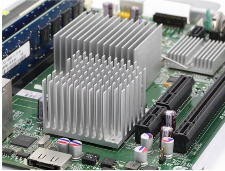
Figure 1-1: Finned heat sinks used to cool various devices on a motherboard [5]
