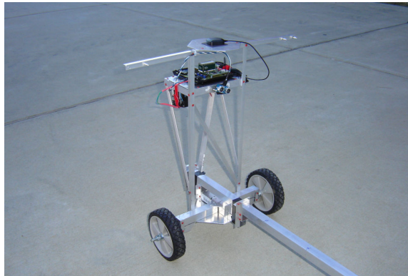
Figure 2.14: Test Rig used to replicate Trail UGV
