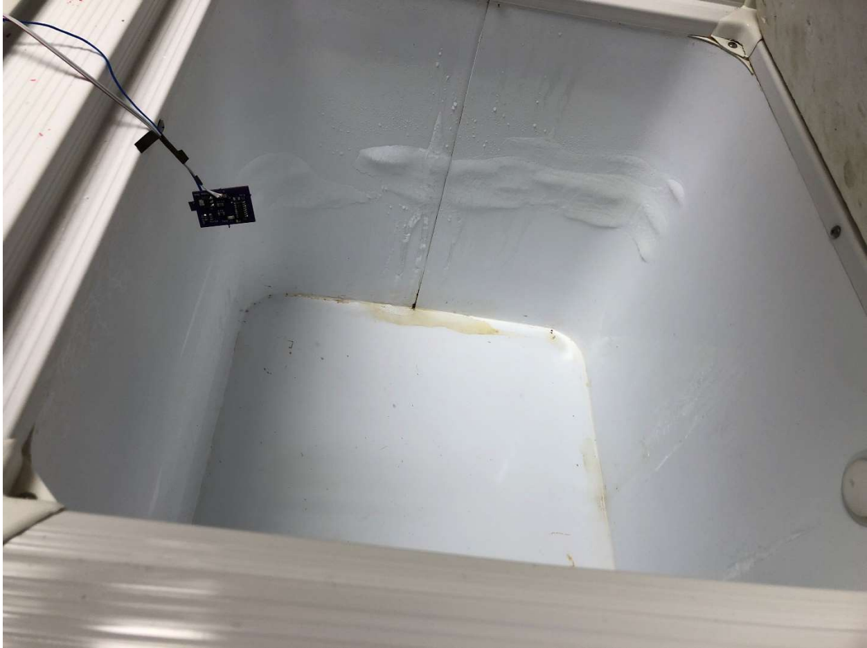
Figure 4.1.2: Thermistor Sensor Board inside Freezer
