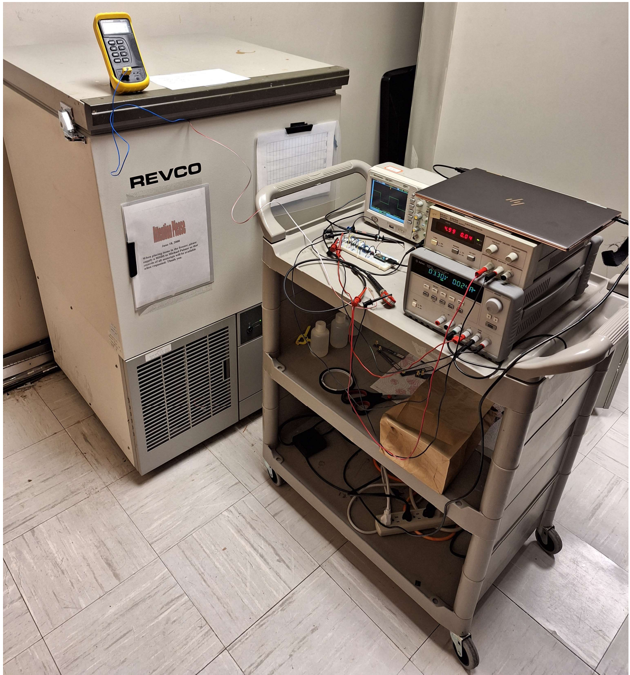
Figure 4.1.1: Thermistor Interface Circuit Test Setup
