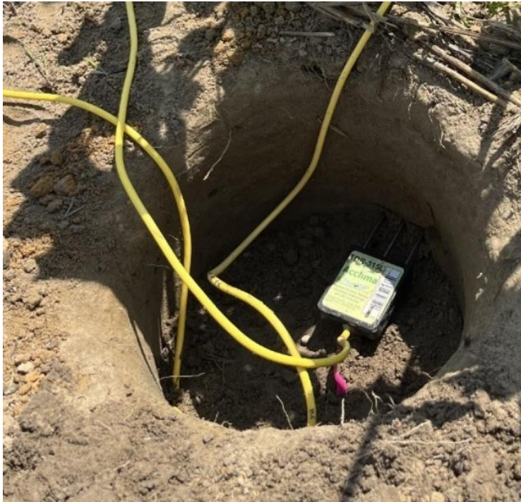
Figure 0.4 Acclima TDR-315H sensor used for collection of real-time soil moisture data.
