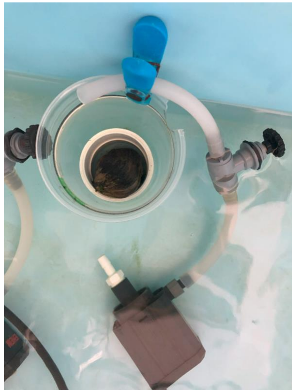
Figure 1.2. Diagram of respiration chamber with associated pumps (top) modified from Haney et. al 2019. Filtration chamber and associated pump for measuring clearance rate (bottom).
