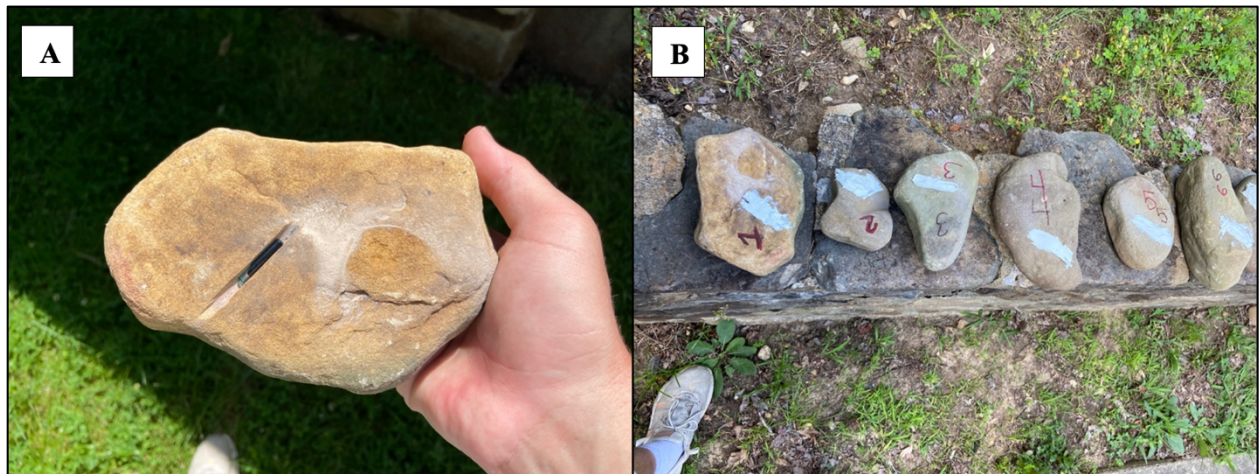
Figure 3.2: Preparing cobbles for the RFID tracer experiment in Beech Creek. Each cobble was indented with a portable angle grinder and fitted with a passive-integrated transponder (PIT) tag (A) and water-resistant epoxy (B).
