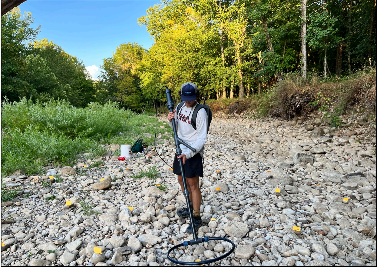
Figure 3.4: Utilizing the OregonRFID equipment in the field. Tagged objects are passively identified via emitted radio waves from the antenna to the tag and vice versa. The antenna communicates with the GNSS receiver and then transmits location-based data to the reader, which can then be downloaded and analyzed.
