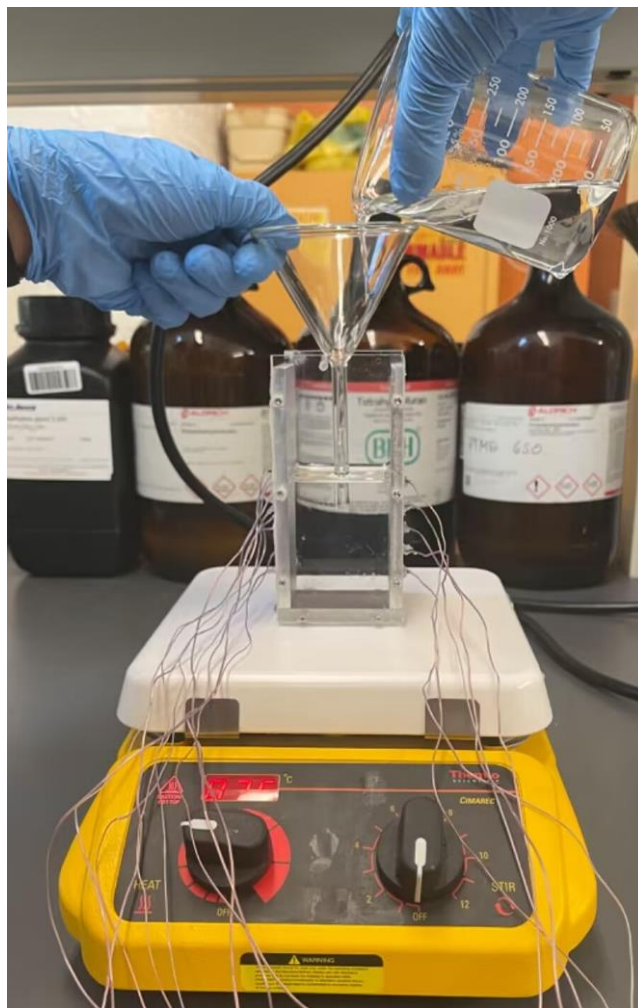
Figure C.2: Pouring the PCM
