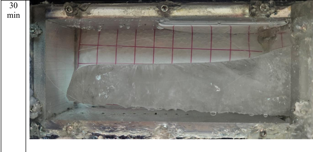
Figure 4.10: Instantaneous progression of the liquid-solid interface on the front observation window of the set-up during Melting Without Vibration for the inclination angle of 0 degrees (vertically-oriented heated plate on the far left)
