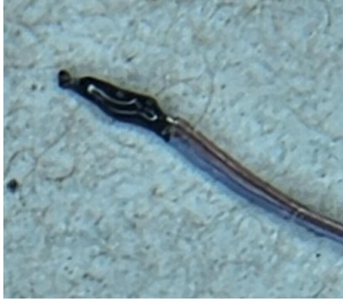
Figure A.8: Thermocouple Head Sealed with Epoxy
