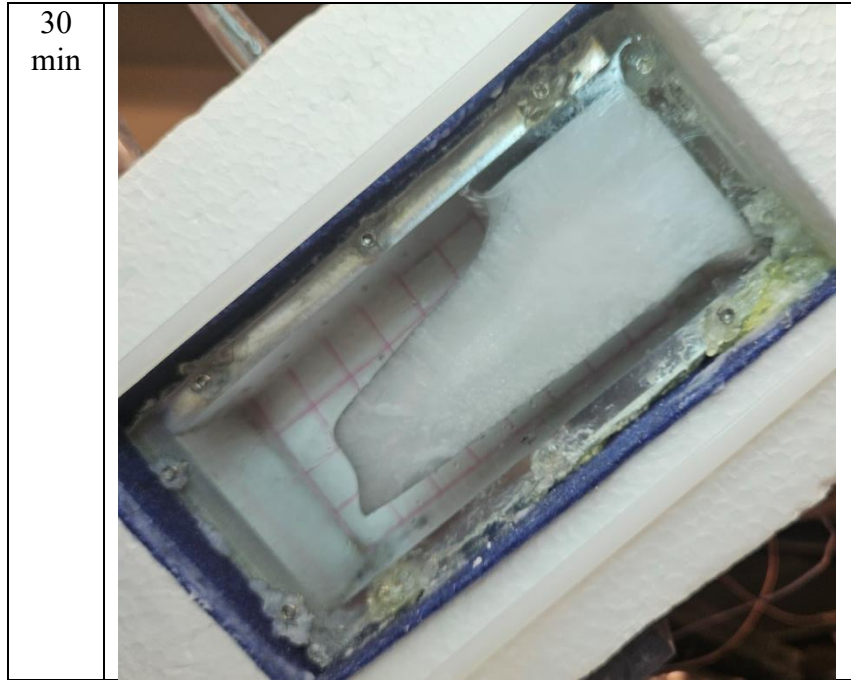
Figure 4.6: Instantaneous progression of the liquid-solid interface on the front observation window of the set-up during Melting Without Vibration for the inclination angle of 45 degrees
