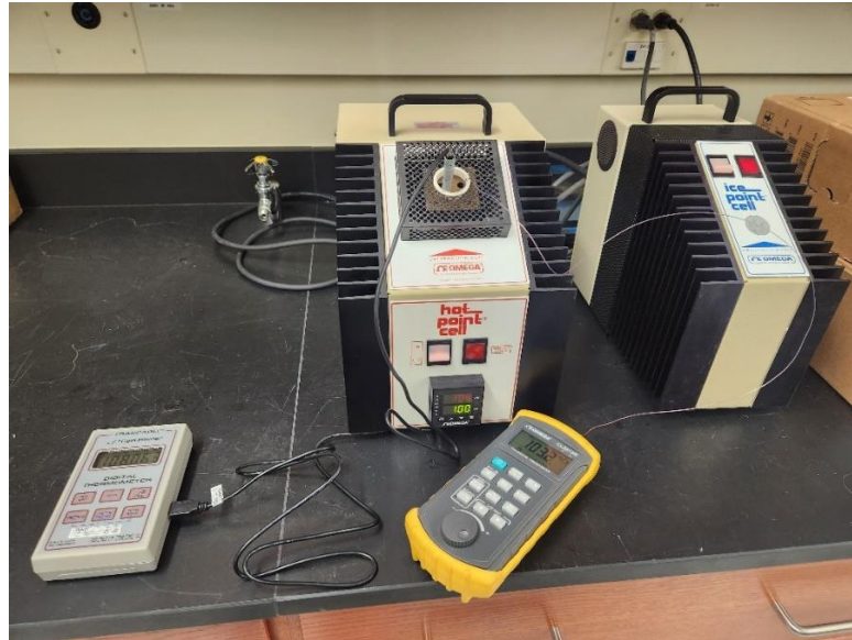
Figure A.7: Testing with Ice point and Hot point Cell
