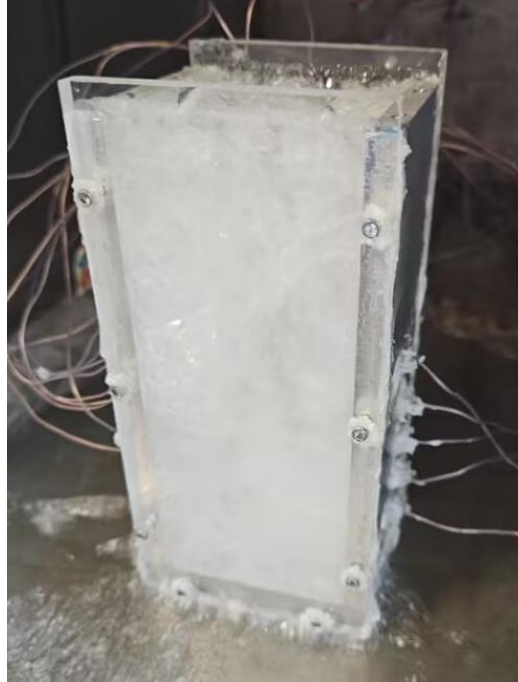
Figure C.6: PCM Pouring Process Done
