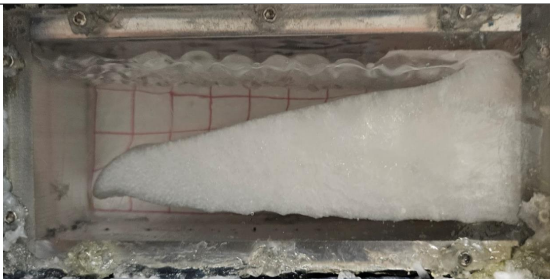
Figure 4.16: Instantaneous progression of the liquid-solid interface on the front observation window of the set-up during Melting Without Vibration for the inclination angle of 0 degrees with Mechanical Vibration at 50 Hz (1G) (vertically-oriented heated plate on the far left)
