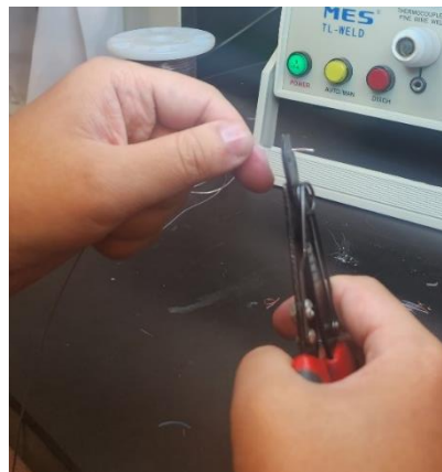
Figure A.2: Stripping the Insulation with the Wire Stripper
