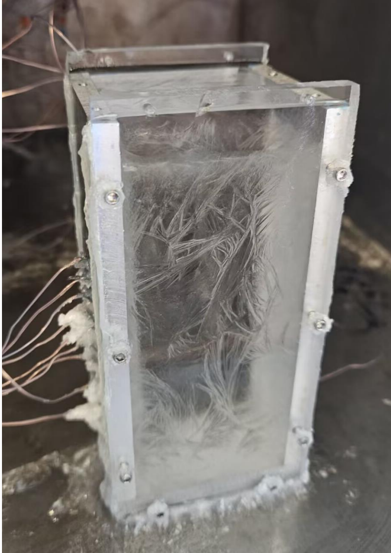
Figure C.7: Solid PCM When Using Step Down Cooling
