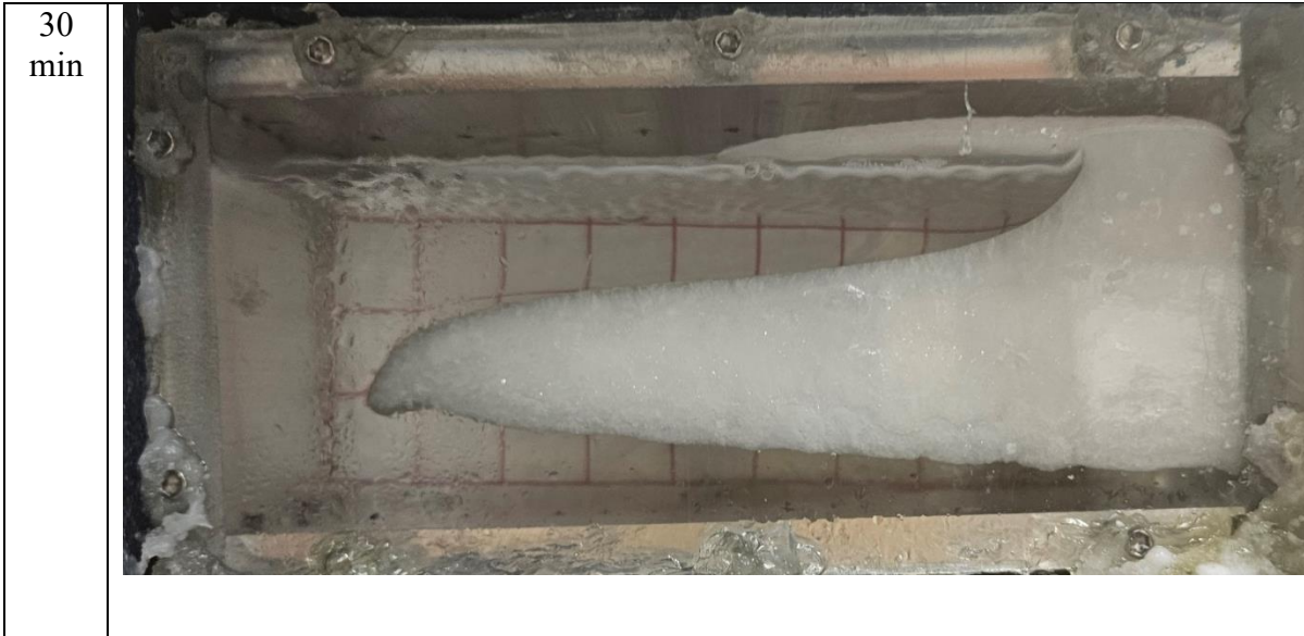
Figure 4.18: Instantaneous progression of the liquid-solid interface on the front observation window of the set-up during Melting Without Vibration for the inclination angle of 0 degrees with Mechanical Vibration at 100 Hz (1G) (vertically-oriented heated plate on the far left)
