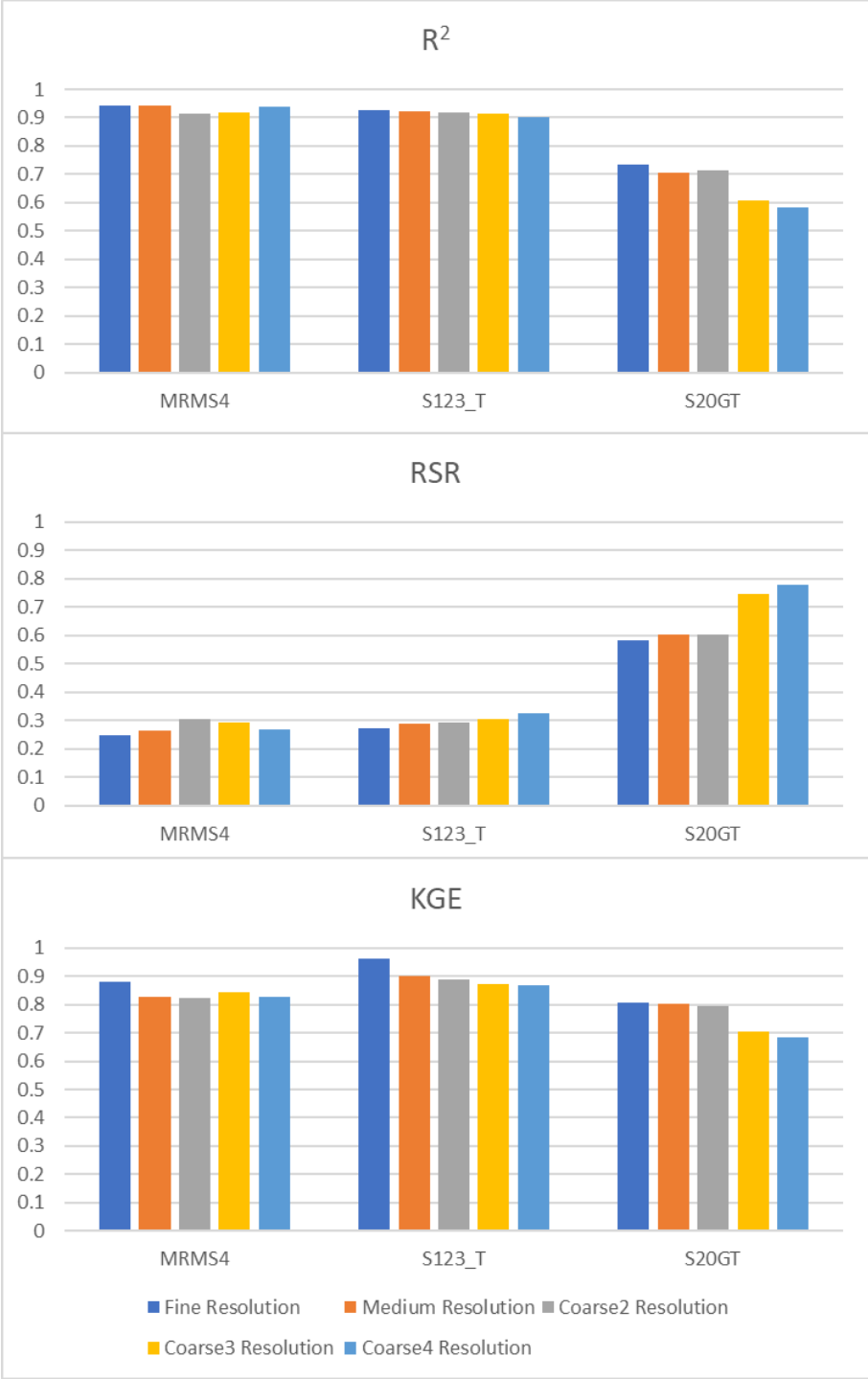
Figure 7: Bar chart illustrating the statistical indicators comparing measured and modeled WSE across the different resolutions and stations.
