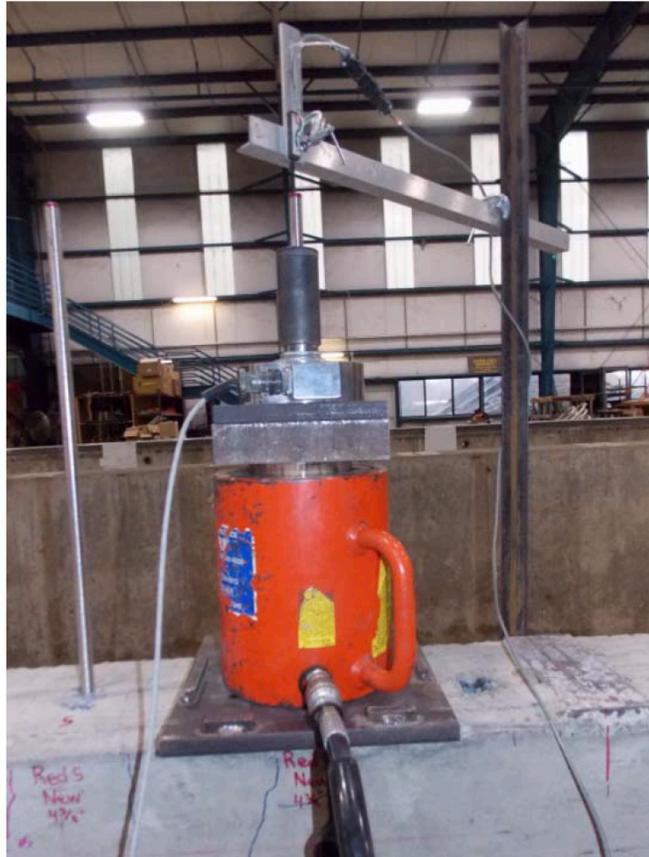
**Figure 2.10 - Pull-out test (Barker, 2014)**
