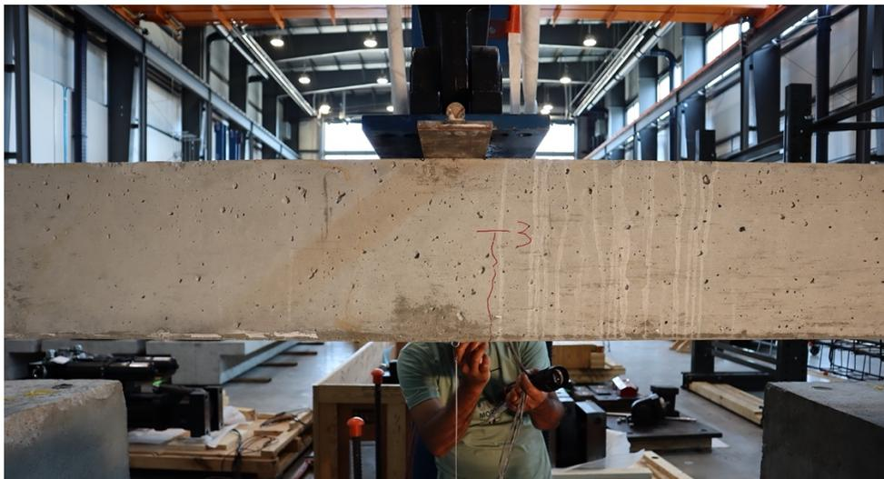
**Figure 7.2— Crack initiation during Pre-Cracking**
