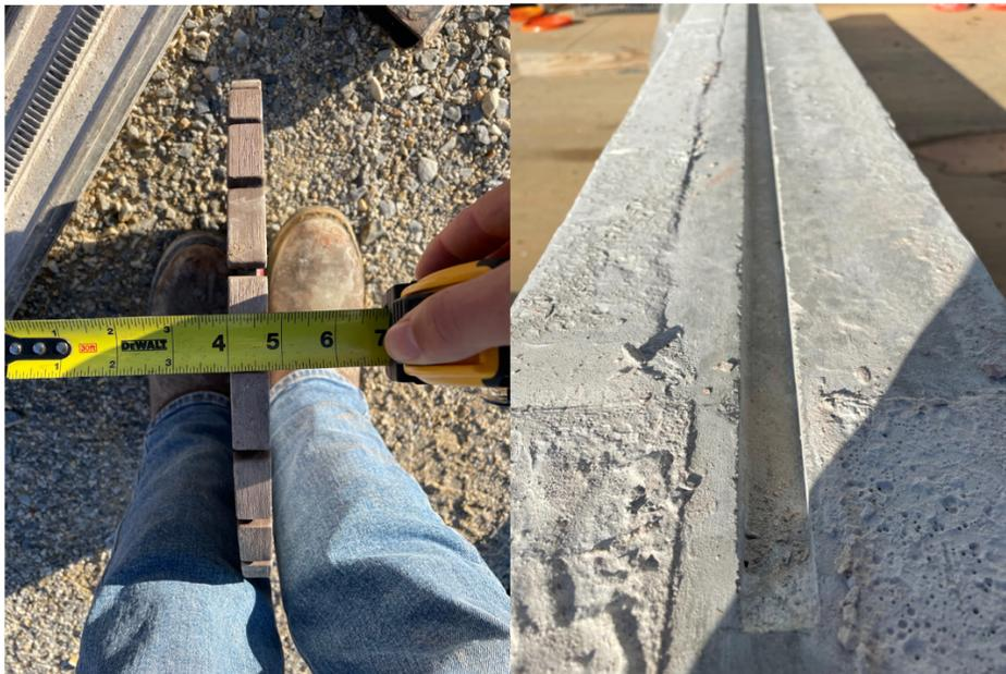
**Figure 7.6-- Custom 0.75 in. wide blade and Corresponding Groove**
