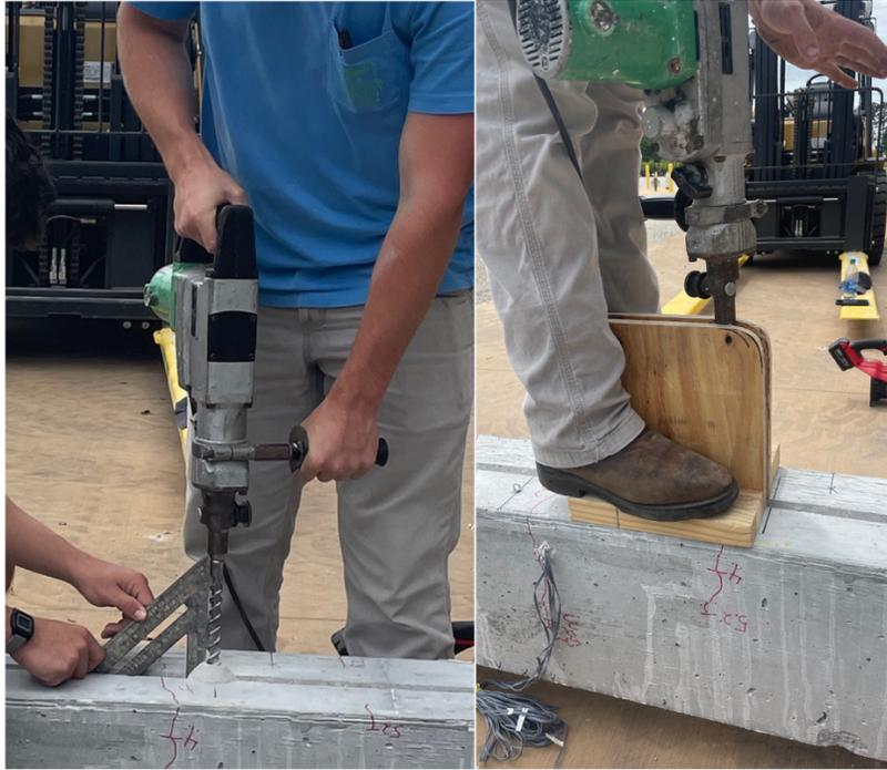
**Figure 7.8— Hammer drill used for Hole (Left) and Bevel (Right)**
