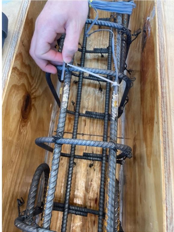
**Figure 6.6— Strain Gauge on Tension Steel**
