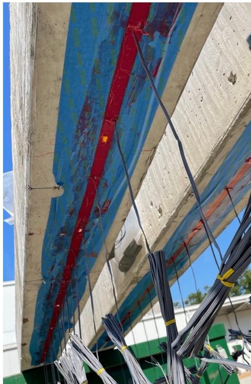
**Figure 7.13— Installed TiAB after Final Epoxy Lift**
