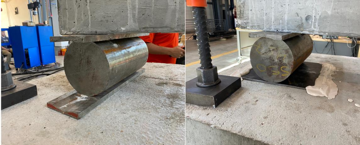
**Figure 6.2— Pin Support (left) and Roller Support (Right)**
