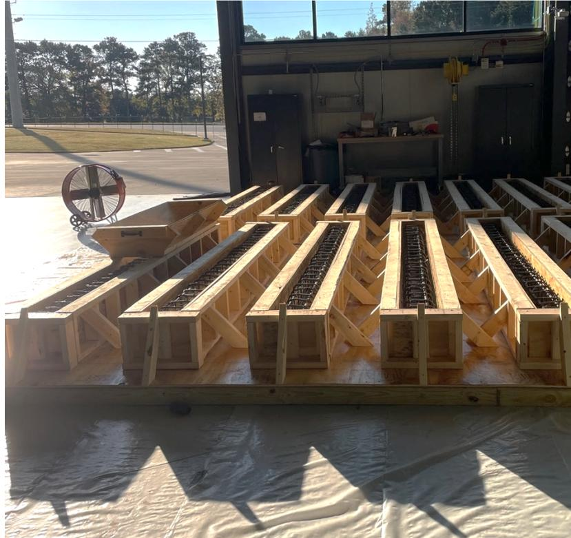
**Figure 5.7— Concrete Forms and Sliding Funnel**
