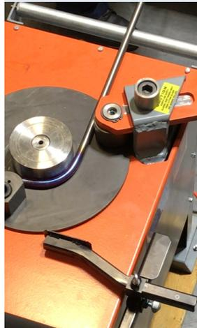
6.9.2 If one end already has a hook, direction of bar and flatness will be critical. Ensure that hook lays on flat surface while bending the other hooked end.
