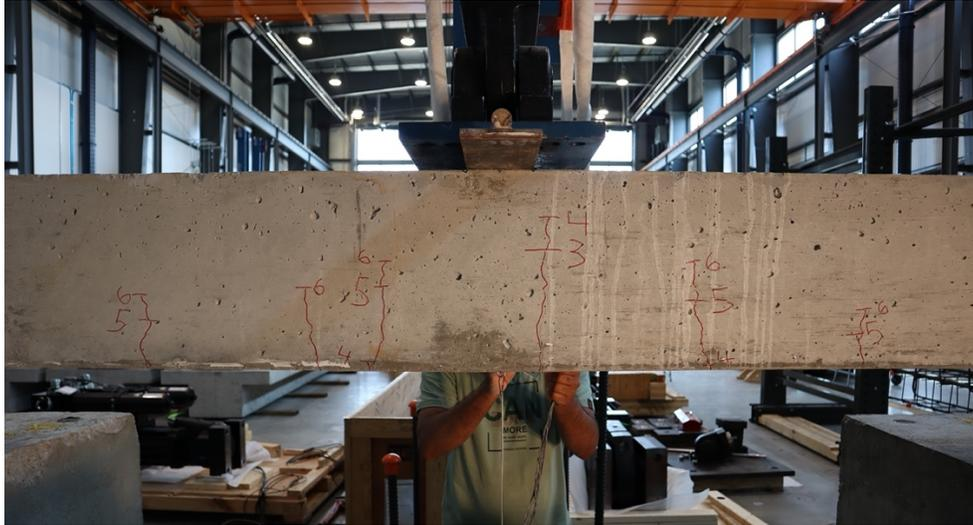
**Figure 7.3— Typical Crack Pattern at end of Pre-Cracking**
