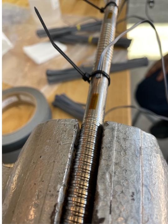
**Figure 6.8— Strain Gauge attached to TiAB**
