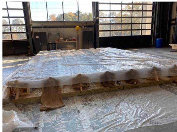
**Figure 5.10 – Beams after Placement (Left) and During Curing (Right)**
