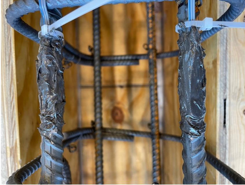
**Figure 6.7— Strain Gauges with Polysulfide Coating**
