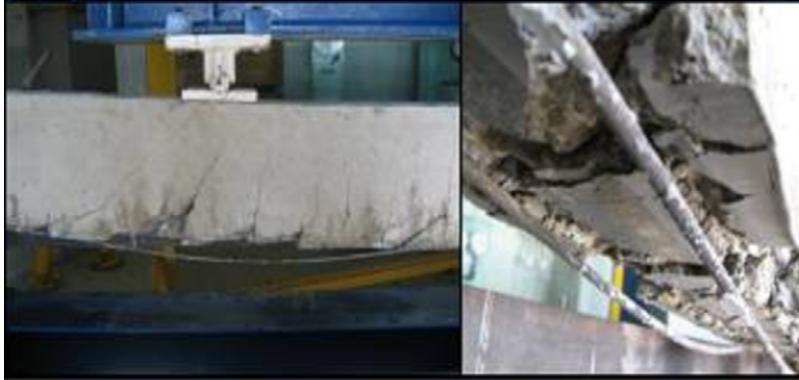
**Figure 2.16 – Epoxy Rupture (Al-Mahmoud, et al. 2009)**
