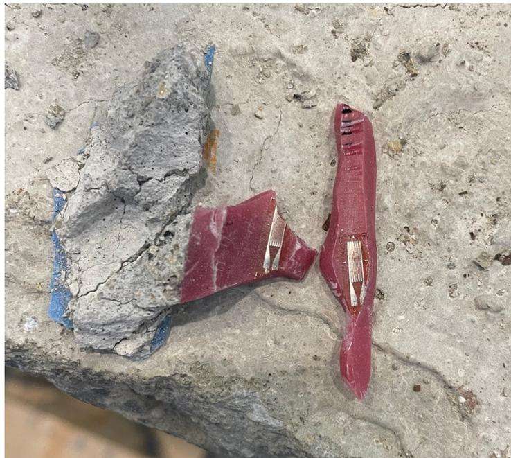
**Figure 6.5 – Strain Gauges and Epoxy Post-Test**
