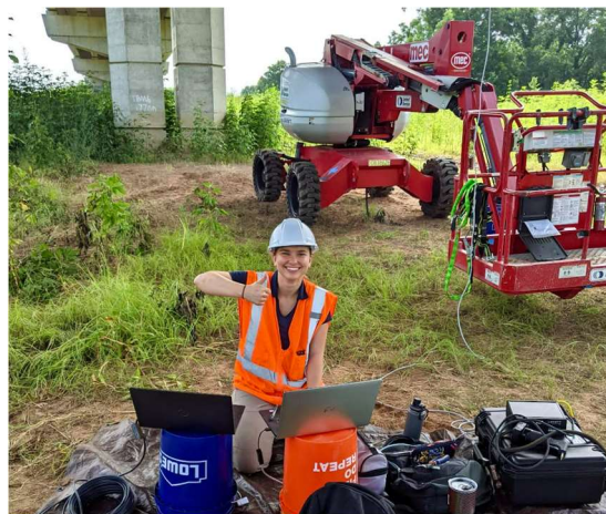
Figure 6-16. Sensor Monitoring During Loading
