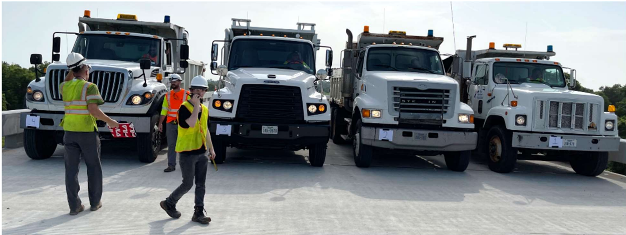
Figure 6-18. Truck Setup for SH 105 Bridge Load Case #1
