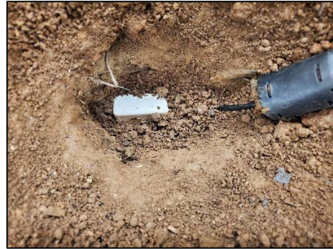
(b) Water volume content sensors installed in topsoil
