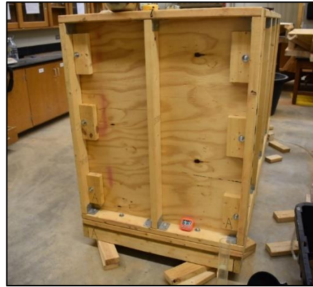
(b) Infiltration swale chamber assembled
