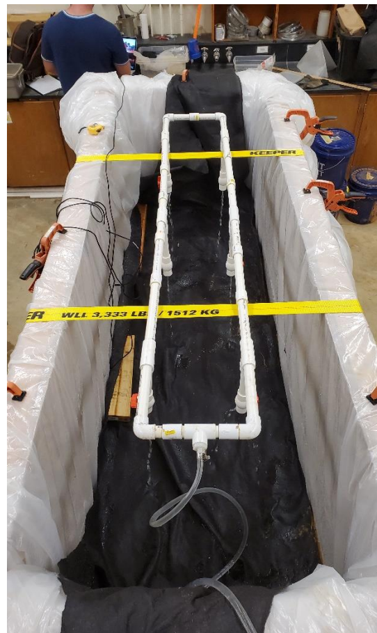
(b) Sand consolidation on infiltration swale chamber
