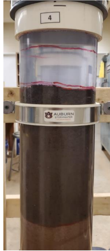
(b) Settlement on amended topsoil layer after all tests
