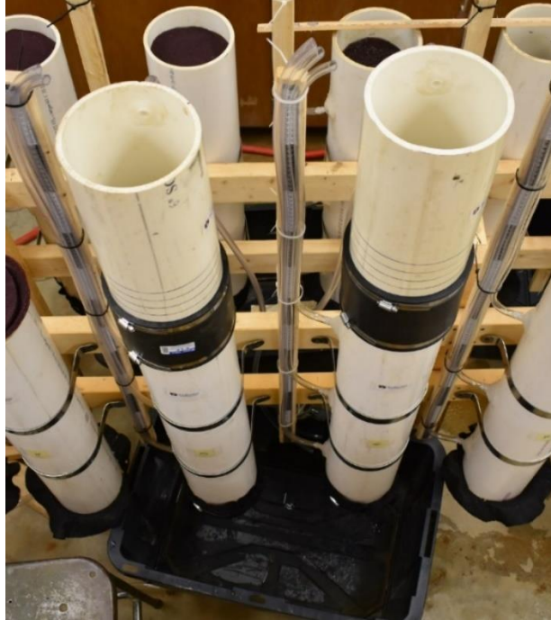
(b) Plastic tote to collect water during the test
