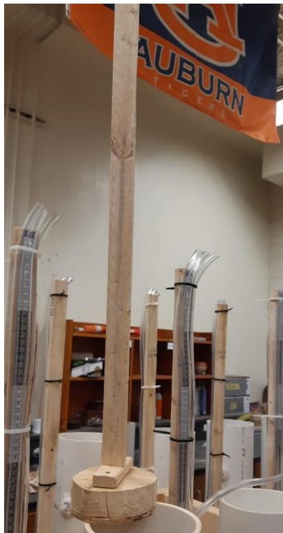
Figure 3-19. Manual Wooden Rammer Designed to Compact Materials.
