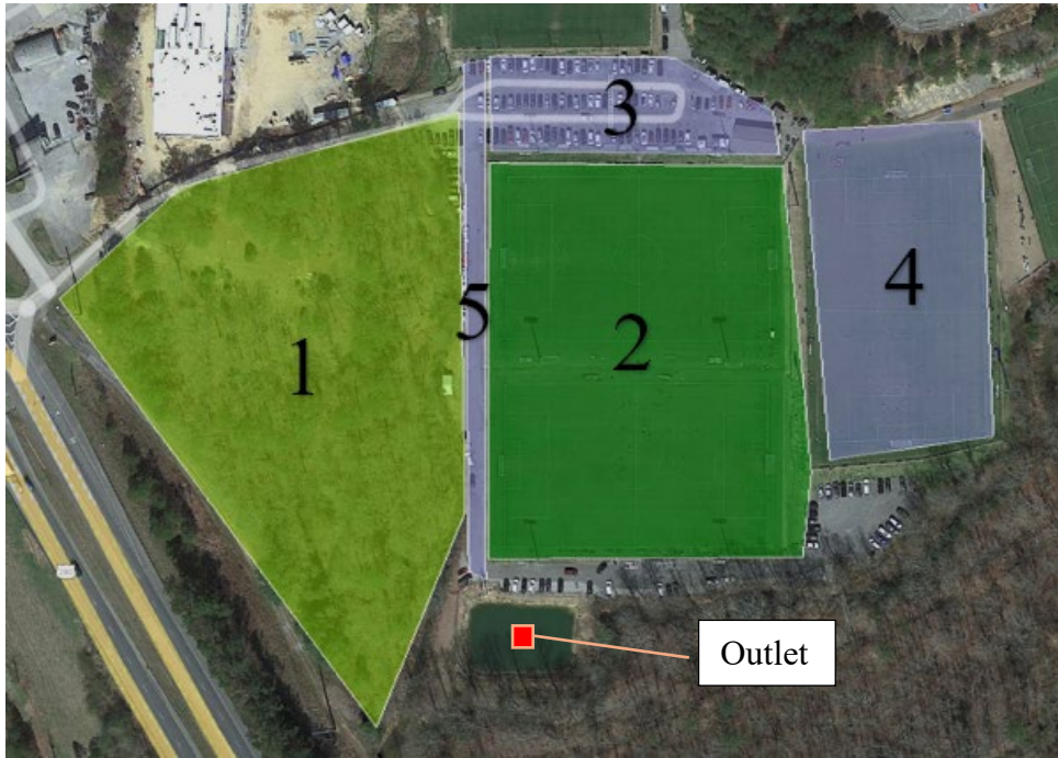
Figure 20: Birmingham site of a soccer field with parking lot and forested area. All runoff is conveyed to the rectangular detention facility in the south edge of the drainage area.
