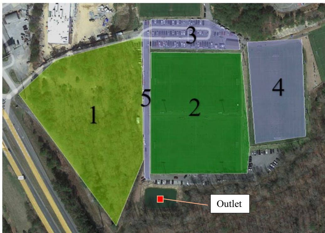
Figure 8: Site division of sub-areas. All runoff is conveyed to the rectangular detention facility in the south edge of the drainage area.
