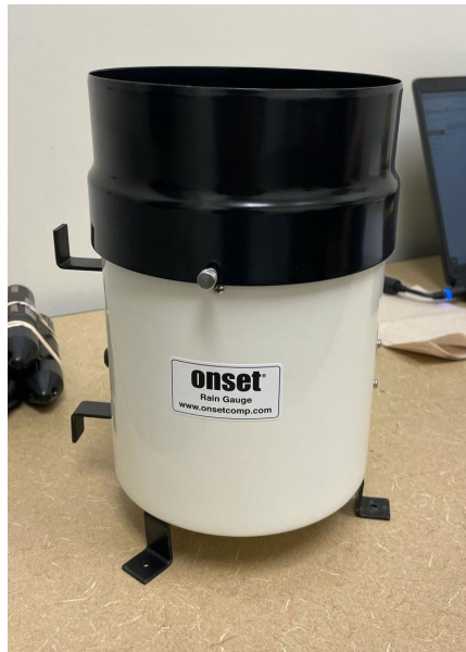
Figure 1: A rain gauge with a tipping bucket.
