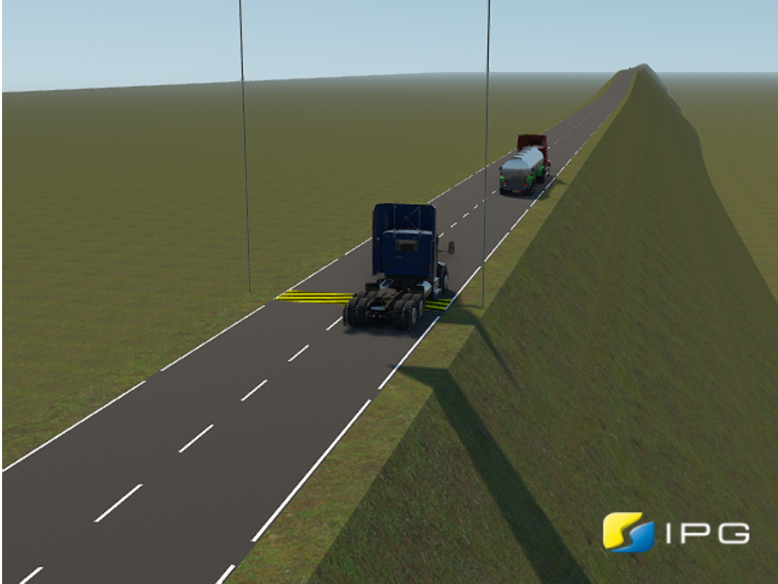
Figure C.2: Screenshot of the vehicle simulation as it passes the 1 km mark and begins the simulated grade.
