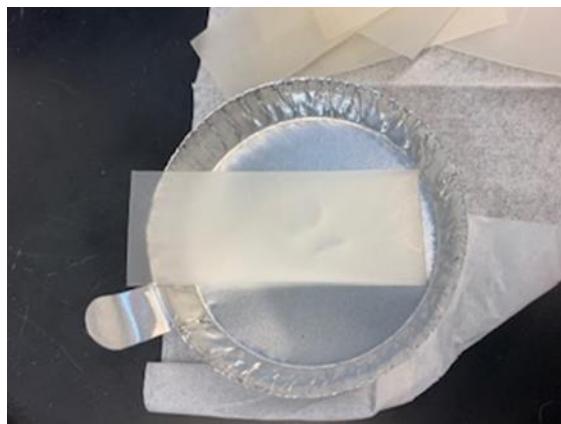
Figure 8: 3.02 cm x 7.62 cm roughened polypropylene bacteria enumeration strip in aluminum pan.
