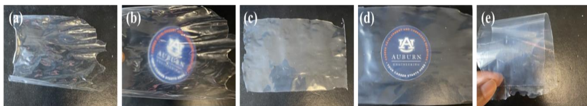
Figure 2.7 (a,b) Pure CNC film cast at 20 s -1 shear rate (thickness: 35 μm) and (c,d,e) Pure CNC + NaCl films cast at 20 s -1 shear rate (thickness: 25 μm)
