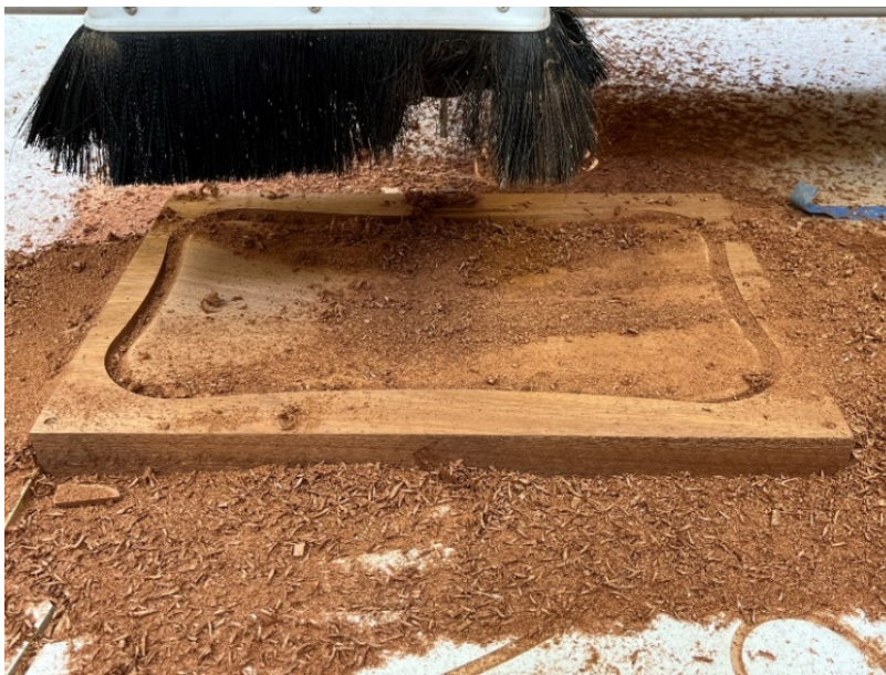
Figure 5.24 Carving process of the seat surface.
