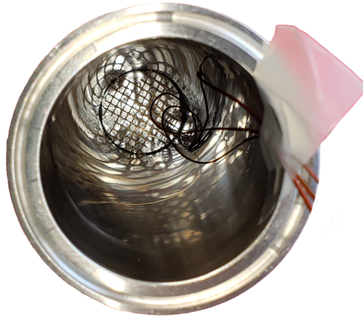
Figure 2.11: Placement of first thermocouple support in microfibrinous media bed.
