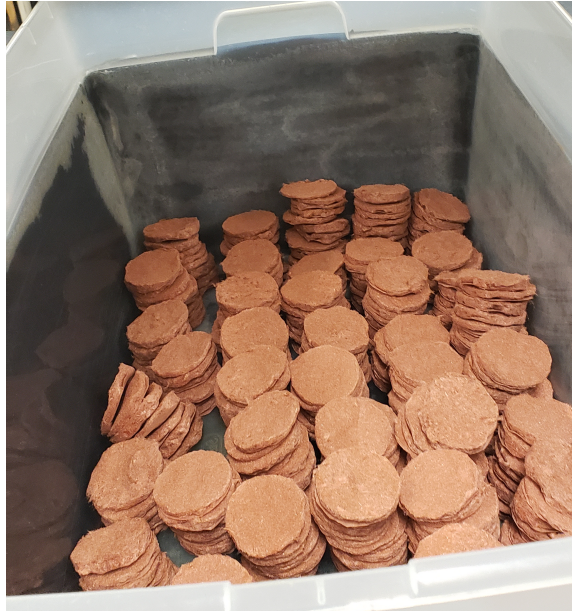
Figure 2.12: Microfibrous media that has been cut but not compressed stored in a plastic tub.
