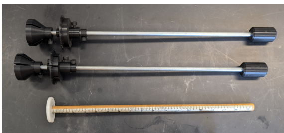
Figure 2.5: Tools used for loading packed beds. Two slotted push rods with head diameters of approximately 58.7 mm with caps that can be clamped to a 3.5-inch sanitary flange and stop collars with thumb screws; these push rods will be referred to as clamping push rods. One push rod with a head diameter of approximately 55.5 mm.
