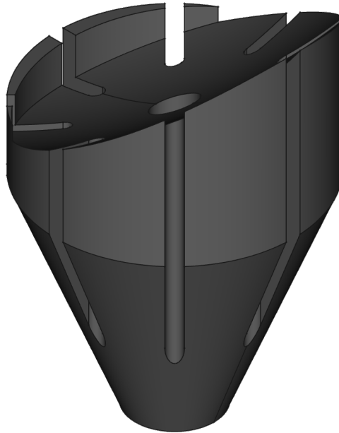
Figure 2.10: Slotted concave push-rod head with a diameter of approximately 59.5 mm.
