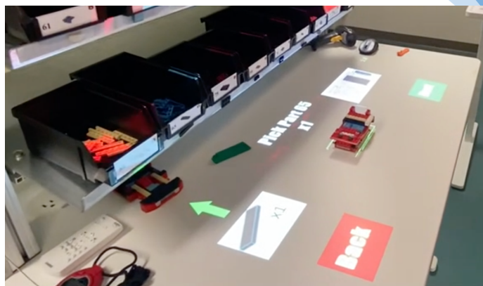
Figure 5- LightGuide Work Instructions
