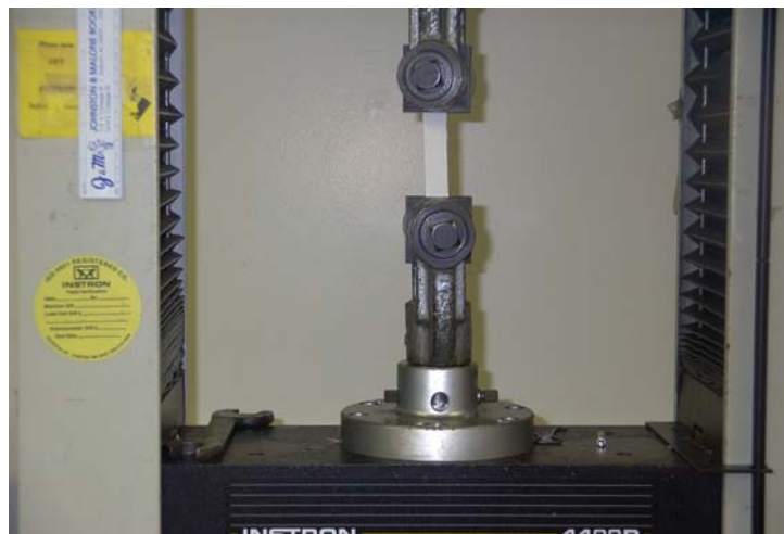
Figure 3.15: Experimental arrangement for tubular woven samples on Instron (machine direction)
