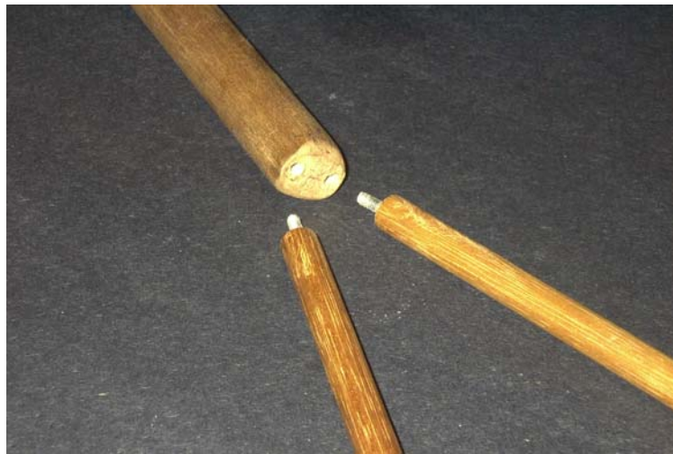
Figure 3.9: Dismantled wooden mandrel used for braiding bifurcated stent
