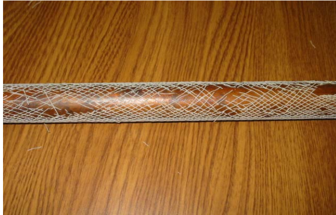
Figure 4.3: Degradation of braided sample at 226 °C (440 °F).
