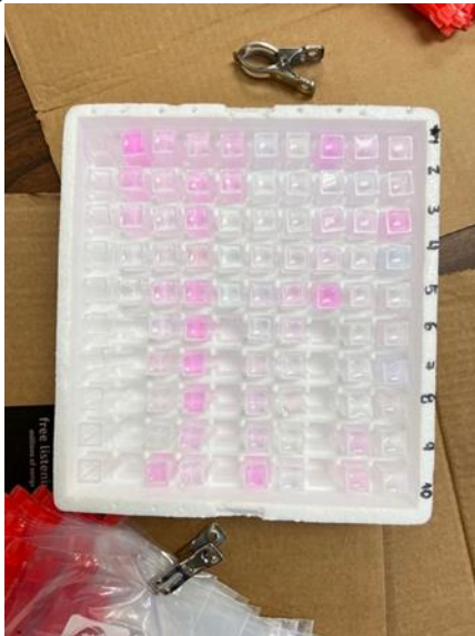
Figure 2. Mylar card and WSP placed in the field (a) and ear leaf (b), extracted fluorescence dye ready for analysis (c), fluorimeter used for dye analysis, detection limit was 1 ppb.
