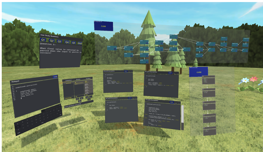
Figure 4.4: VR Enhanced representative screenshot showing the default components (notepad, question control, main menu) and additional items spawned and arranged by the user: four text slates, a function call graph, and a control flow graph.
