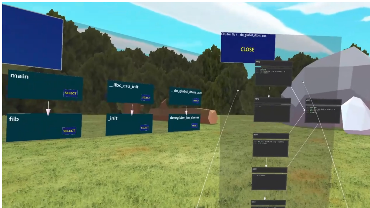
Figure 3.21: Iteration 3 screenshot: a call graph for a simple binary with a control flow graph for one of its functions; darkened area indicates the grabbable area of the graph.
