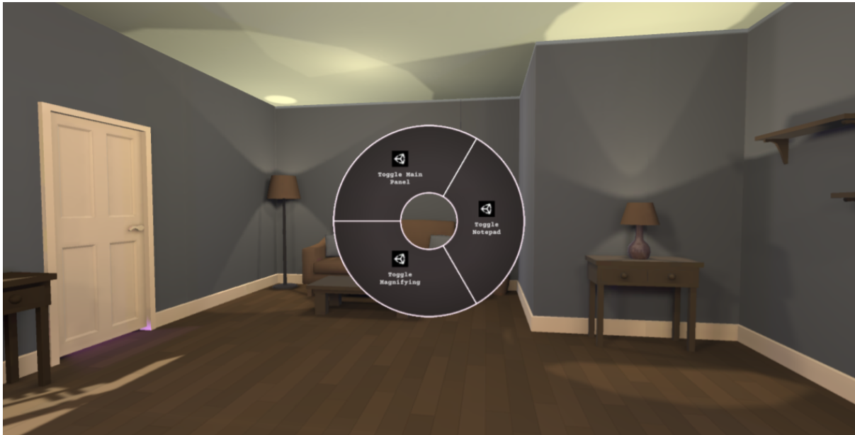
Figure 3.14: Iteration 2 screenshot: the radial menu allows users to enable and disable the main menu, notepad, and magnifying glass from the touchpad of the VR controller.
