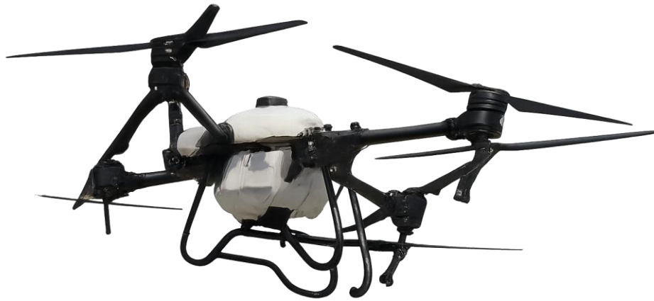
Figure 3. The DJI Agras T40 drone sprayer used in the spraying experiments.
