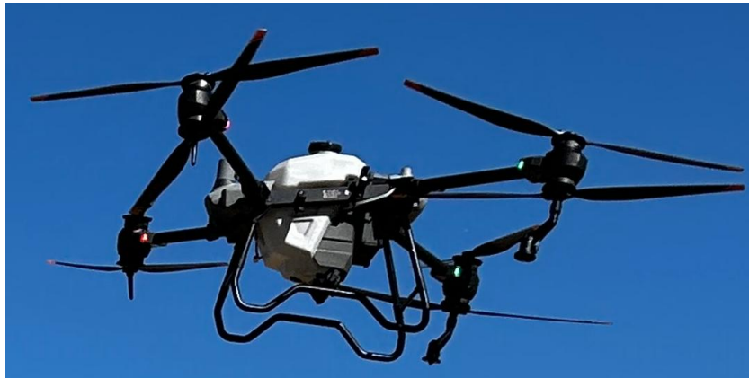
Figure 12. DJI Agras T40 drone sprayer used in the spraying experiments.
