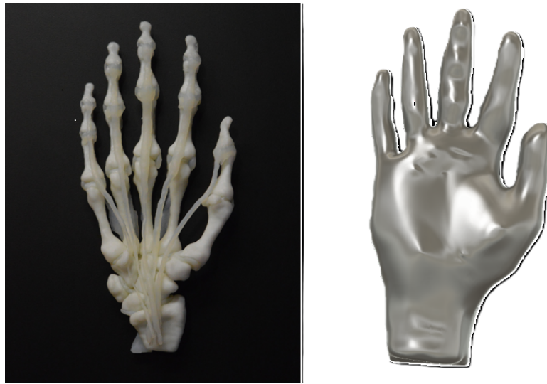
Figure 2.7: Axial 3D’s hand model printed with the J5 Digital Anatomy Printer is depicted on the left, and the corresponding digital representation of the external morphology of the hand derived from the same MRI scan generated in 3DSlicer is presented on the right.
