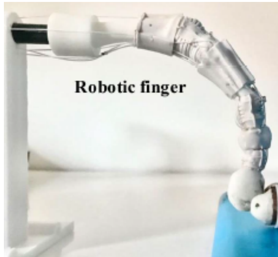
(c) Zhu et al. used polyethylene terephthalate (PET) fiber ribbons to simulate ligaments and thin high-density capsules that were sintered to bone across joints. Tendon sheaths were created with silicone rubber and fibers with fishing line (figure reproduced from [14]).
